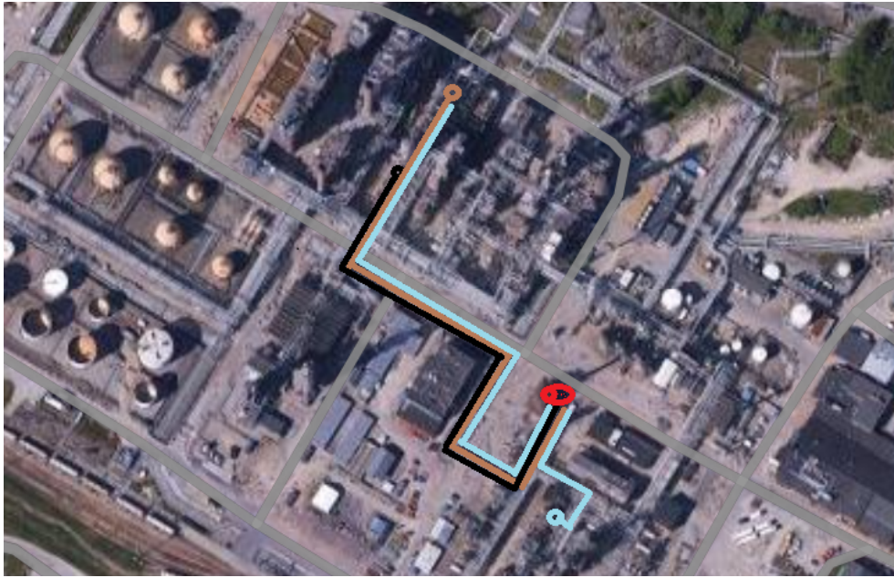
Figure 5.13: Position and piping for the AHT. The brown line is the overhead, the black one is quench oil and the blue one is the stripper water. The red circle is the possible position of the AHT.
