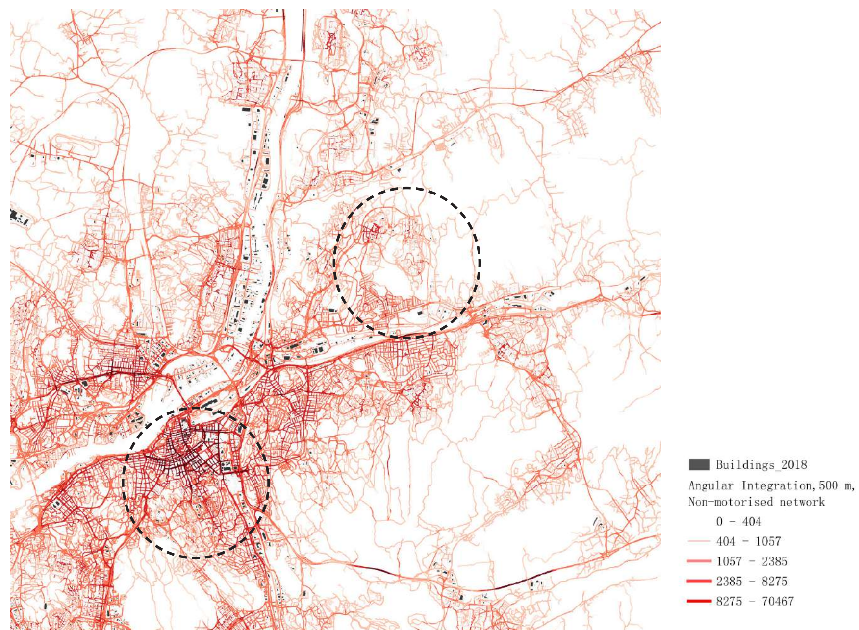
Figure 12. Network centrality and angular integration analysis in Bergsjön. Produced by author using QGIS, 2026.
