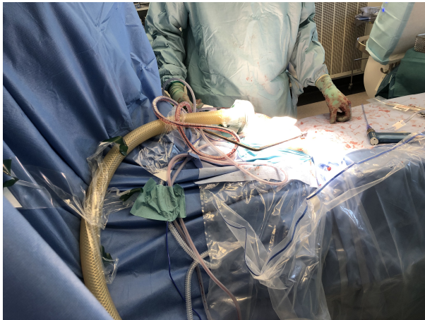
Figure 12: Sample head and tube placed within 30 cm from the surgical wound for the active sampling measurement.
