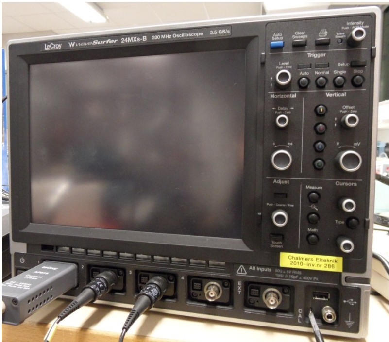
Figure 49: Picture of the LeCroy 24MXs-B Oscilloscope used to get the readings from the probes and to calculate the input power.
