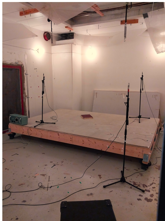
Figure 7: Measurement setup in the reverberation chamber.
