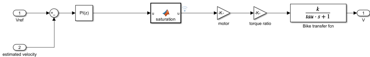
Figure A.1: Simulink model of the speed controller.
