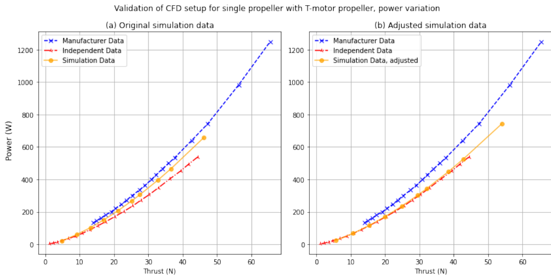
Figure 4.6: Validation of thrust for T-motor propeller against power change
