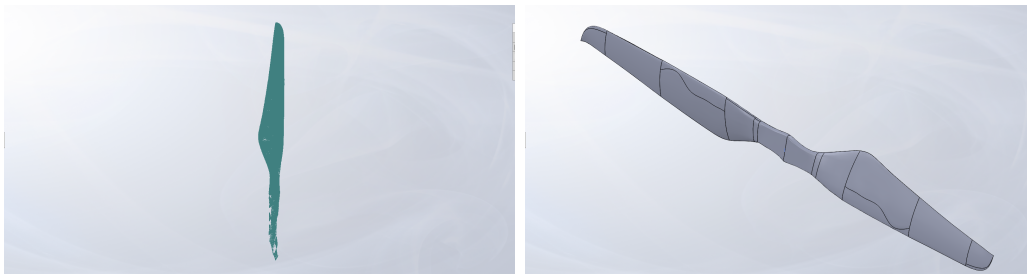
(a) 3D Point cloud scan of propeller (b) Scanned propeller CAD model
