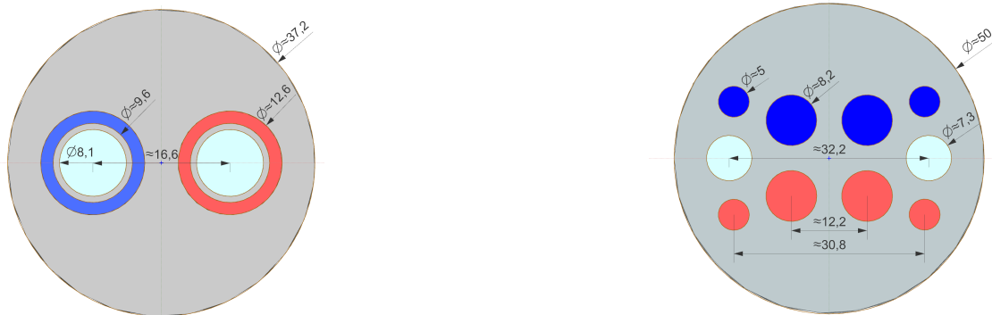
Figure 3.5: Water-cooled cable models: (a) Type One (copper-clad water integration), (b) Type Two (separate cooling channel design).
