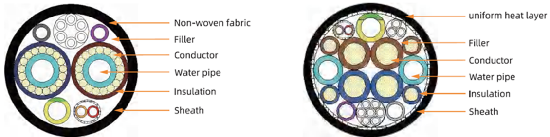
Figure 3.3: Water-cooled cable structures: (a) type one (copper-clad water integration), (b) type two (separate cooling channel design)[9].
