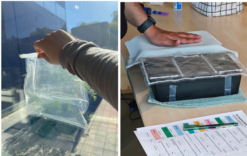
Figure 37: The air-insulated blind: test see-through effect on the window (left) and the evaluation setup (right).
