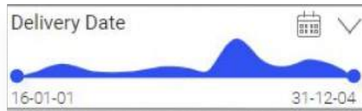
Figure 7.2: A closer look at the slider for filtering delivery time with a calendar icon that opens up the delivery date dialogue window when the user presses it.
