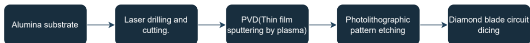
Figure 4.1: Representative thin-film fabrication flow for the probe substrates, shown for process context only.
