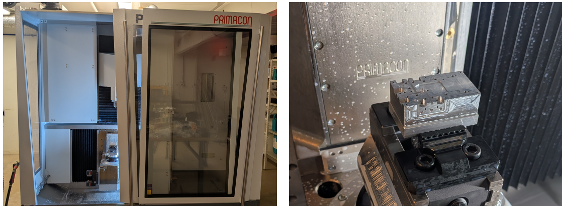
(a) Primacon P40 CC CNC machine (b) Split-block during milling
