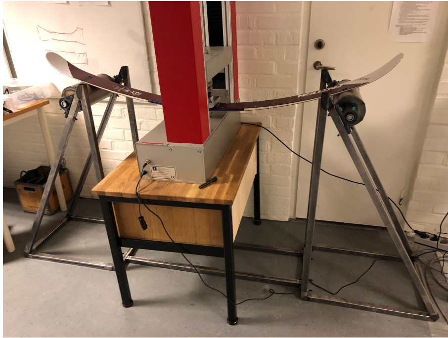
Figure 20: Picture showing the three point bending test on Candide 3.0.
