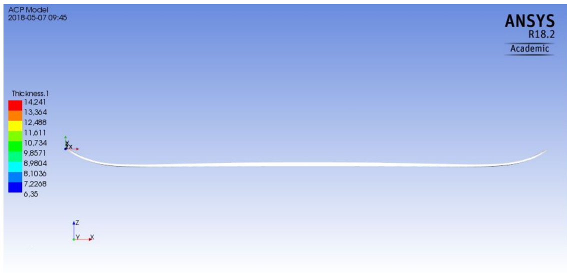
Figure 4: Render of the ski with a variable thickness core and correct geometry.
