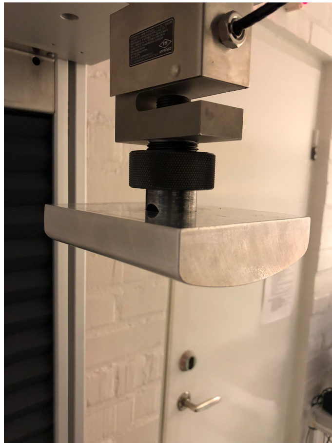
Figure 19: Picture of tool mounted via press fit in the uniaxial compression test machine
