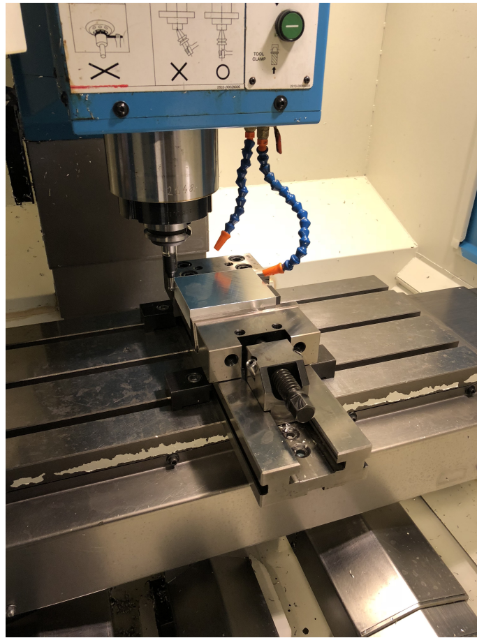
Figure 16: Picture showing the tool mounted in the mill after the first operation.
