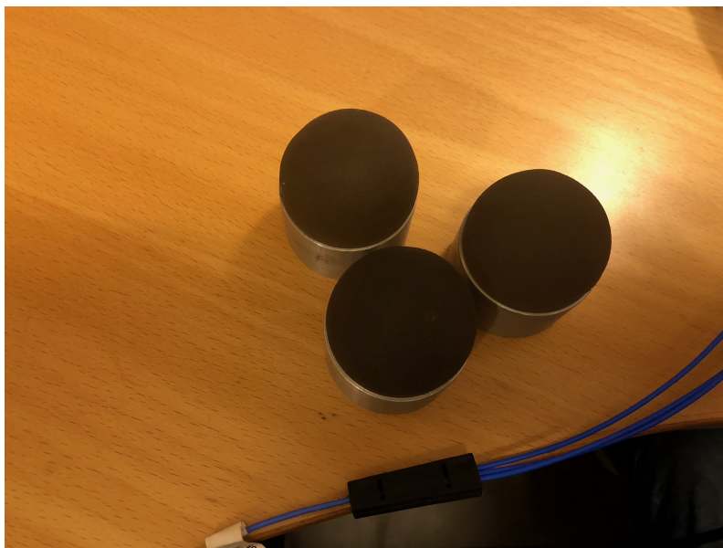
Figure 24: The rubber balls used to isolate the ski during the vibrations analysis.
