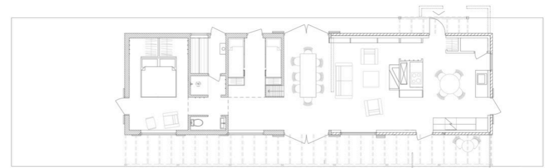
The rather narrow width of the original cabin translates into rooms that really must be uniquely planned to function well well fitting the limited space. Most rooms are placed in line after each other.
