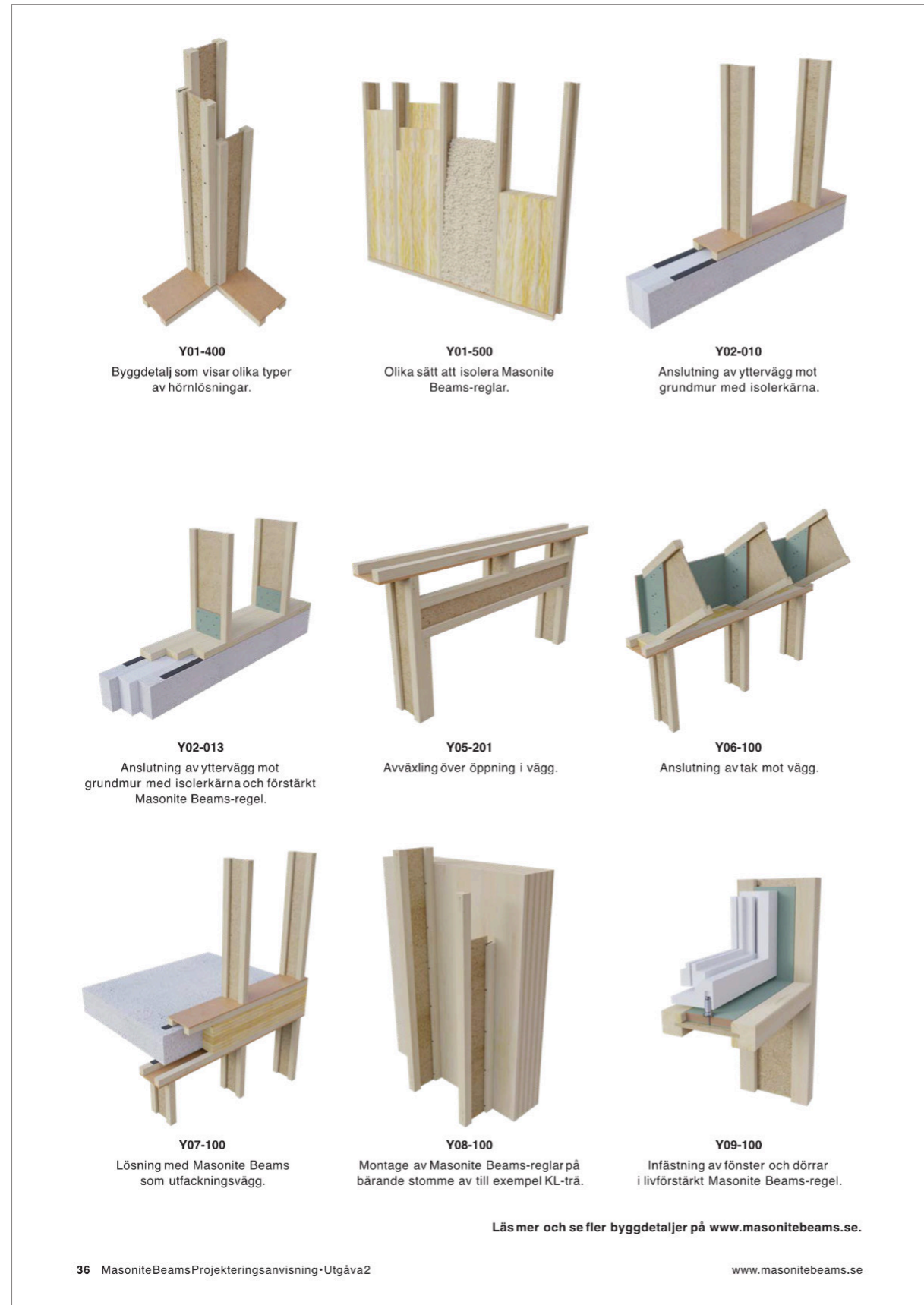
Illustration showing examples of the use of Masonite Beams AB version of I-joists.
