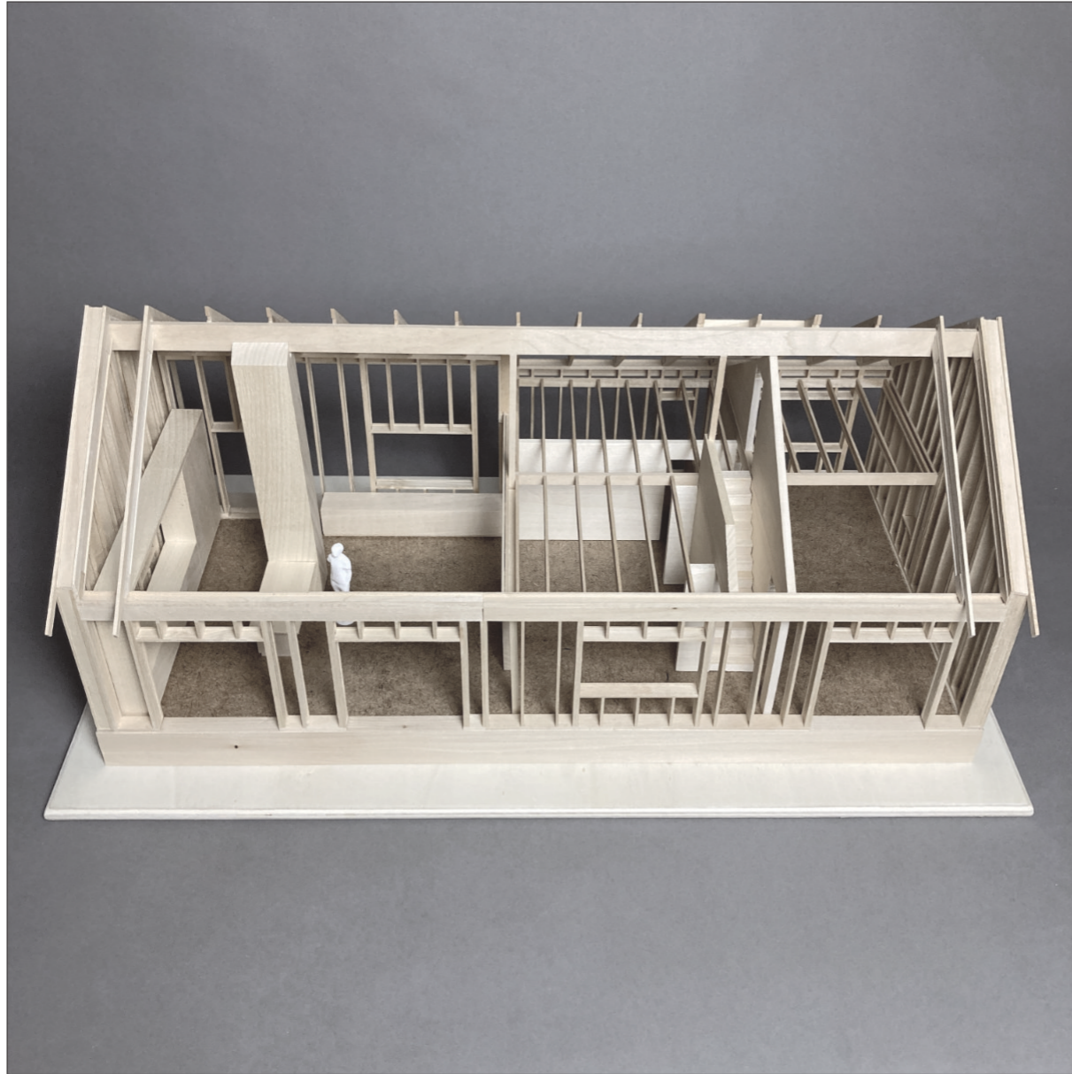
Structural model with interior volumes added - 1:25
