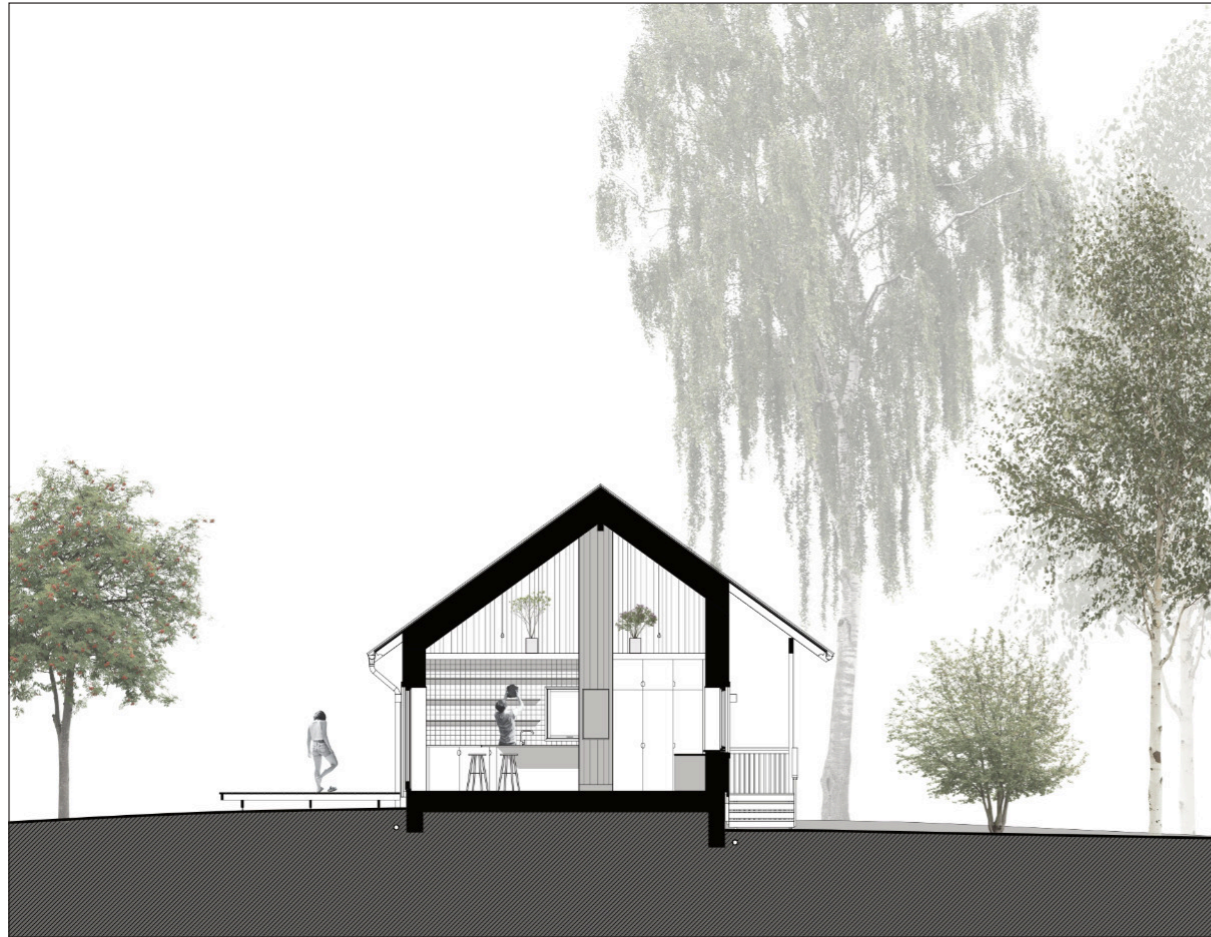
Section B – B, showing kitchen and entrance – 1:150
