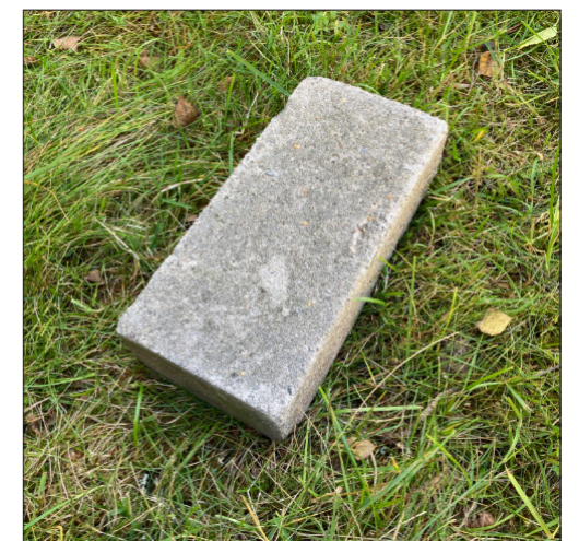
Bricks of concrete was used to lay the chimneys.
