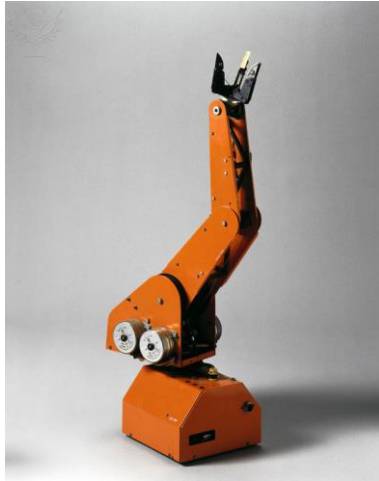
Figure 10 A 5-axis robot arm similar to those used in the automotive industry. Retrieved from Britannica ImageQuest (n.d.c).
