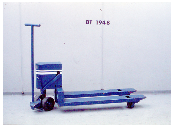
Figure 1.3: BT's hydraulic pallet truck with a swivelling steering column from 1948.
