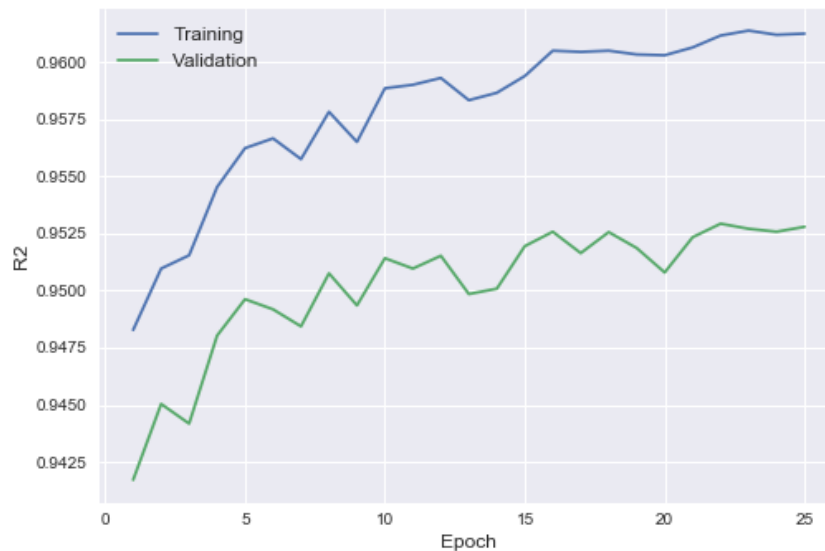
Figure 4.10: A representative example of a typical learning progression, showing the R^2 score during training of MLP version 2. Considering the small gap between the training and validation score, there is barely any presence of overfitting. In this case, the curves indicated that the model could benefit from a longer learning duration, which is why this model was retrained with higher number of epochs.
