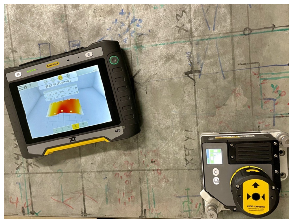
Figure 2.3: Picture shows the deviation of the measured coordinate table with respect to the calibrated reference plane.
