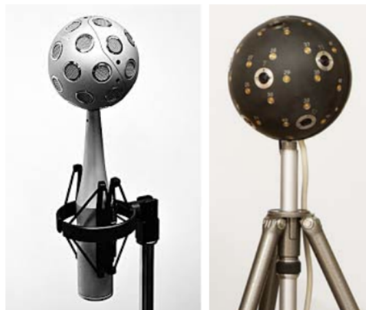
Figure 1.10: Some commercially used spherical microphone arrays. Left: em32 Eigenmike microphone array with 32 channels [23]. Right: BK spherical microphone array with 36-50 channels [15].
