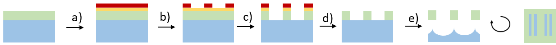
Figure 3.3: An illustration of the chip after each fabrication step. The chip at the start consists of a GaAs layer (blue) and an InGaP layer (green). An adhesion promoter (yellow) and resist (red) is spin-coated to the chip in a). The exposed regions of the resist are then removed in b) by developing. This is followed by dry-etching of the GaAs layer in c). The resist and adhesion promoter is then removed by a remover and hydrofluoric acid, respectively, in d). The resonators are then suspended in e) by wet etch with citric acid and hydrogen peroxide and dried with a critical point dryer.
