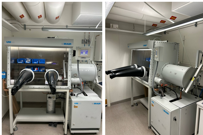
Figure 4.1: Glovebox with argon (99,999%, Linde), used for the mixing of \text{CaH}_2 and \text{BaTiO}_3 .
