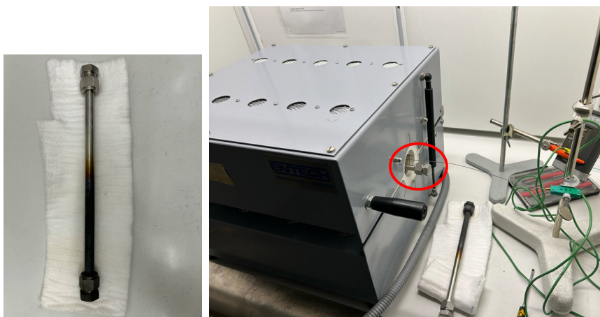
Figure 4.2: Stainless steel capsule (after use) used for \text{BaTiO}_{3-x}\text{H}_y synthesis, shown both individually and placed inside the furnace.
