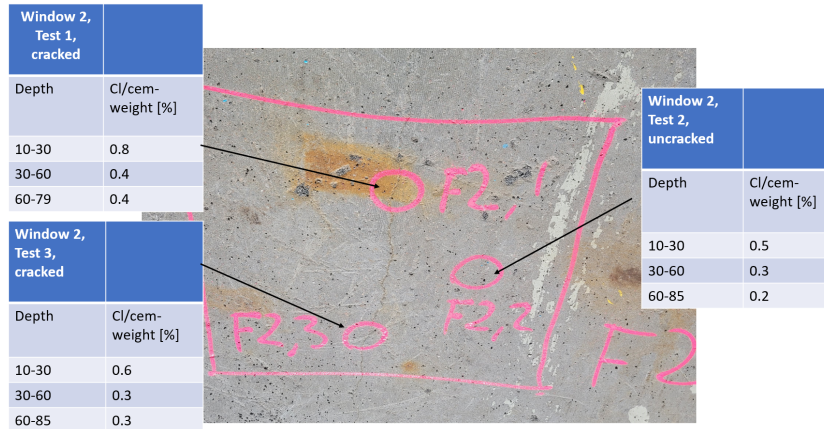
Figure 3.14: Chloride content through depth in window F2 from Afry reports.
