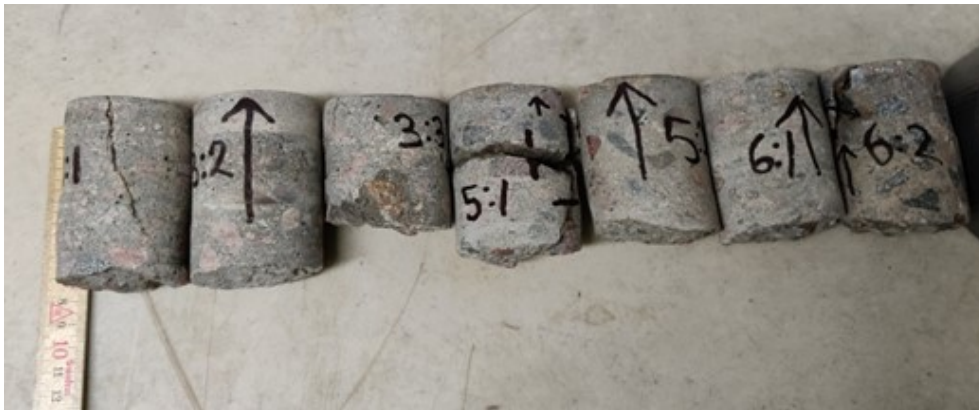
Figure 3.11: Crack width in different samples from Afry reports.
