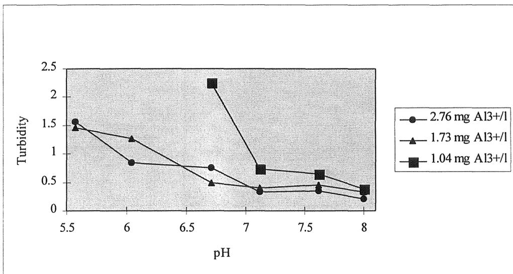
Figure C:4 Effect of dose and pH using PAX XL-1
