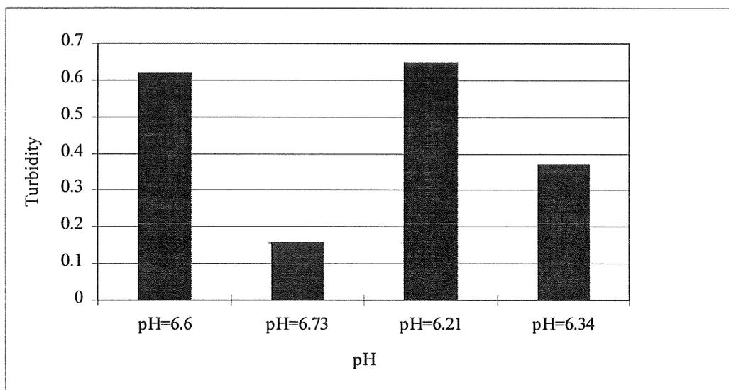
Figure C:10 ALG; Turbidity at around optimum pH, dose 1.73 mg Al<sup>3+</sup>/l, using different samples of raw water
