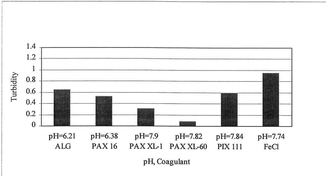
Figure 7:2 Fe-based coagulants compared with PAX XL-1 and PAX XL-60 for unadjusted water. ALG and PAX 16 were added at optimum pH. All coagulants were added at the dose  $1.73 \text{ mg Al}^{3+}/\text{l}$  or  $1.73 \text{ mg Fe}^{\text{tot}}/\text{l}$  and raw water was taken from the same water sample.
