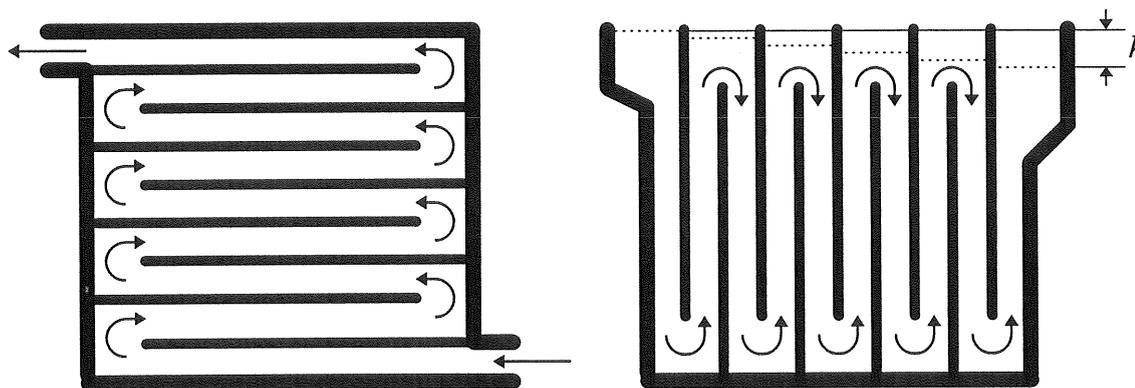
Figure 4:2 Horizontal and vertical baffles
