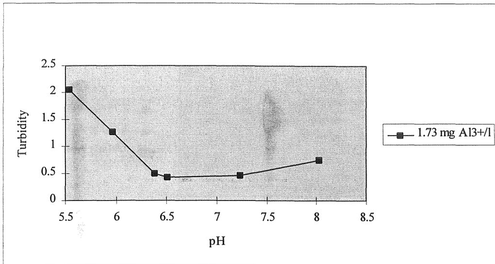
Figure C:3 Effect of pH using PAX 16
