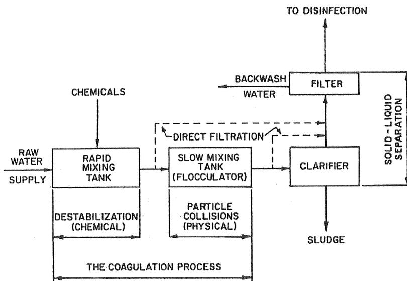
Figure 4:1 Schematic diagram of a coagulation process in a water treatment plant
