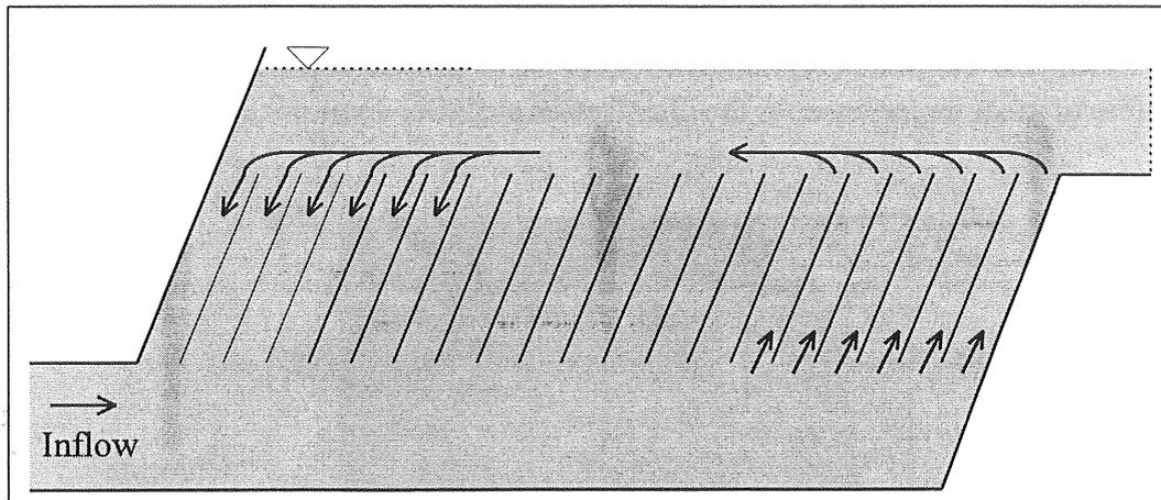
Figure 9:2 Not functional separation in tube settler
