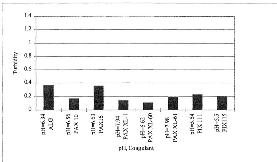
*Figure 7:4 Turbidity at around optimum pH for various coagulants using the same raw water, dose  $1.73 \text{ mg Al}^{3+}/\text{l}$  or  $1.73 \text{ mg Fe}^{\text{tot}}/\text{l}$*
