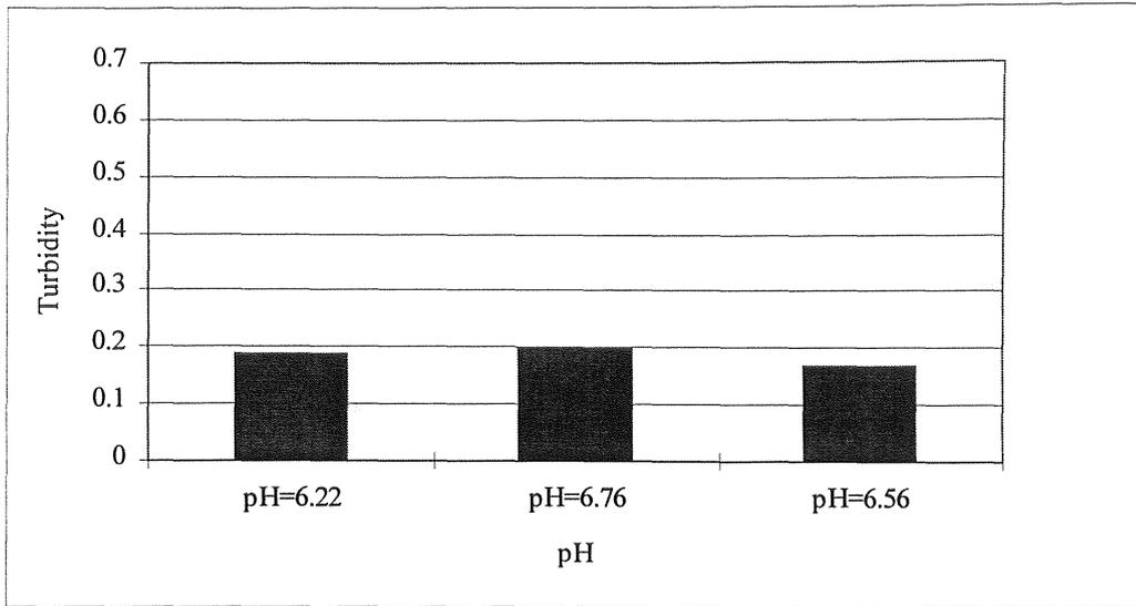
Figure C:11 PAX 10; Turbidity at around optimum pH, dose 1.73 mg  $Al^{3+}$ /l, using different samples of raw water
