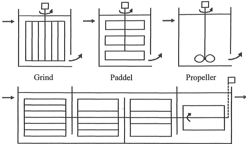
Figure 4:2 Different facilities for mechanical flocculation
