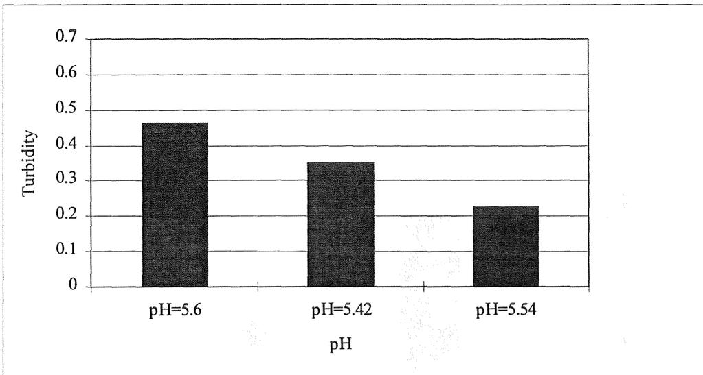
Figure C:16 PLX 111; Turbidity at around optimum pH, dose 1.73 mg Al<sup>3+</sup>/l, using different samples of raw water
