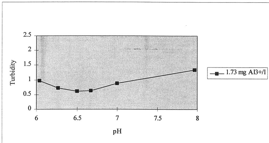
Figure C:1 Effect of pH using ALG
