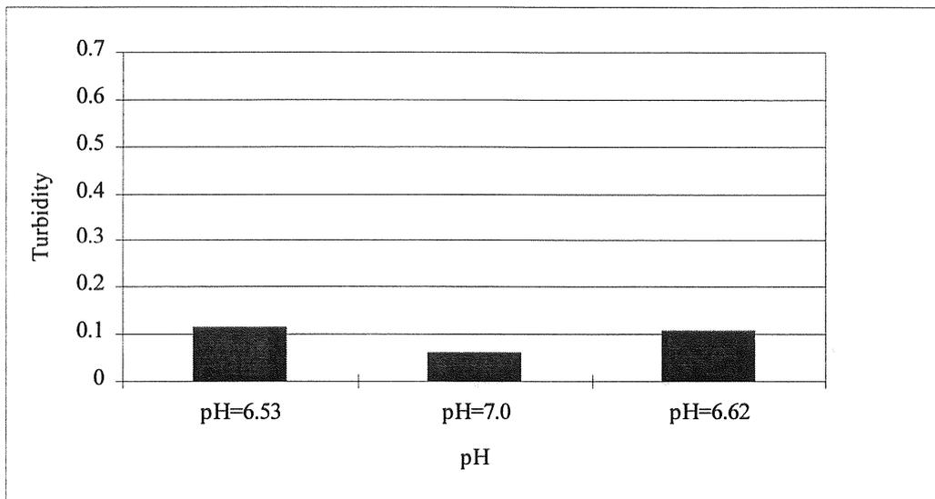
Figure C:14 PAX XL-60; Turbidity at around optimum pH, dose 1.73 mg  $Al^{3+}$ /l, using different samples of raw water
