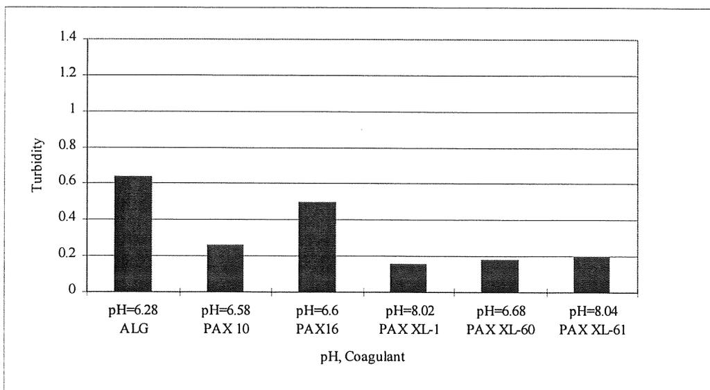
Figure 7:5 Turbidity at around optimum pH for various coagulants using the same raw water, dose 1.04 mgAl<sup>3+</sup>/l
