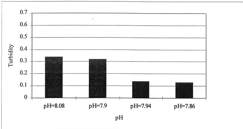
Figure C:13 PAX XL-1; Turbidity at around optimum pH, dose 1.73 mg  $Al^{3+}$ /l, using different samples of raw water
