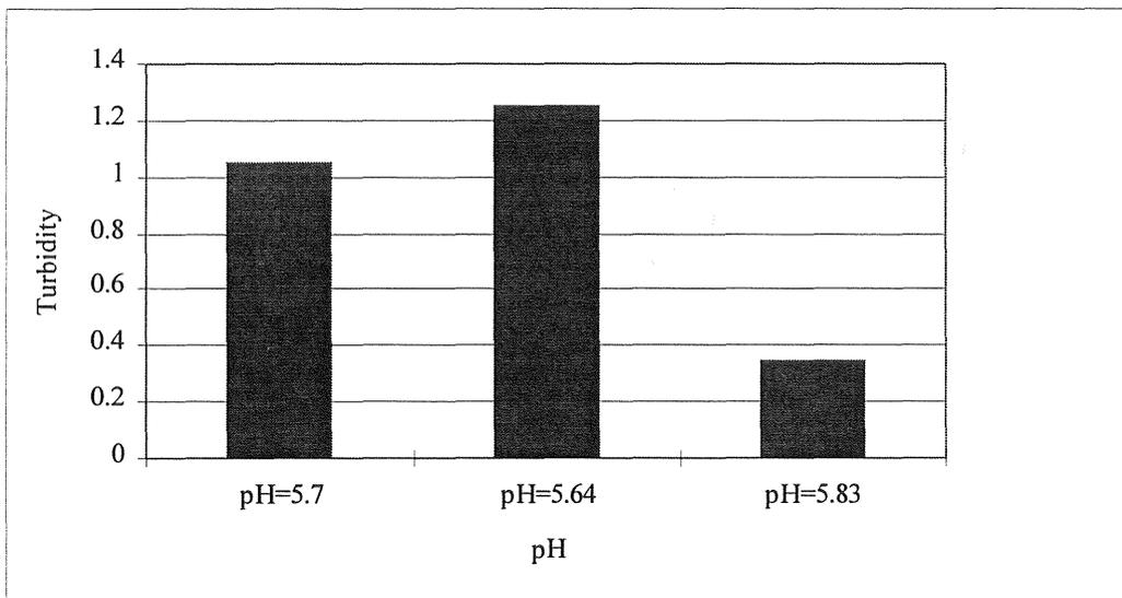
Figure C:18  $FeCl_3$ ; Turbidity at around optimum pH, dose 1.73 mg  $Fe^{tot}$ /l, using different samples of raw water
