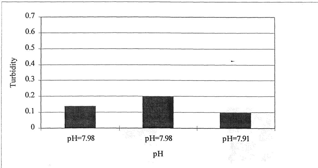
Figure C:15 PAX XL-61; Turbidity at around optimum pH, dose 1.73 mg Al<sup>3+</sup>/l, using different samples of raw water
