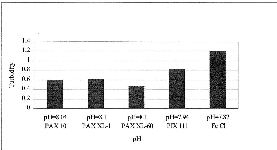
Figure 7:3 Turbidity without pH-adjustment, dose  $0.69 \text{ mg Al}^{3+}/\text{l}$  and  $1.38 \text{ mg Fe}^{\text{tot}}/\text{l}$
