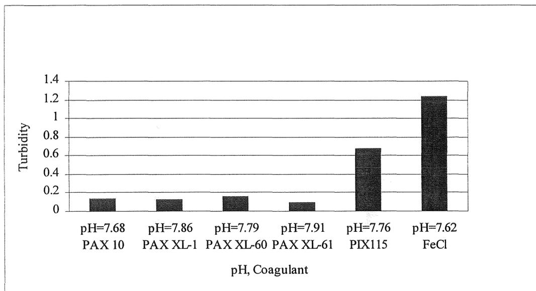
Figure 7:1 Turbidity without pH-adjustment, both Al- and Fe-based coagulants are added using the same sample of raw water at the dose 1.73 mg Al<sup>3+</sup>/l or 1.73 mg Fe<sup>tot</sup>/l
