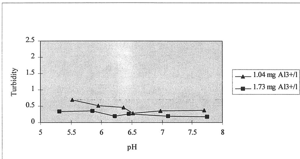
Figure C:2 Effect of dose and pH using PAX 10
