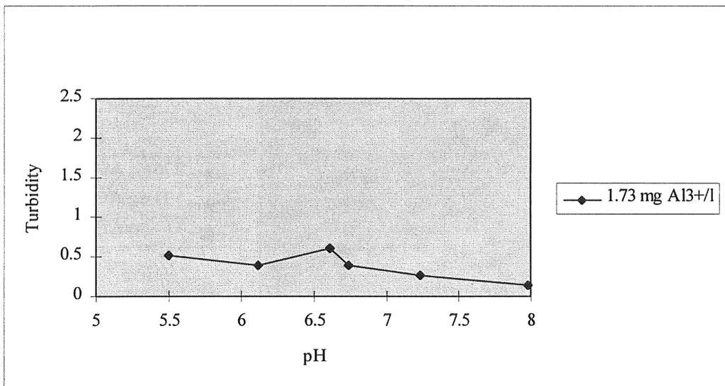
Figure C:6 Effect of pH using PAX XL-61
