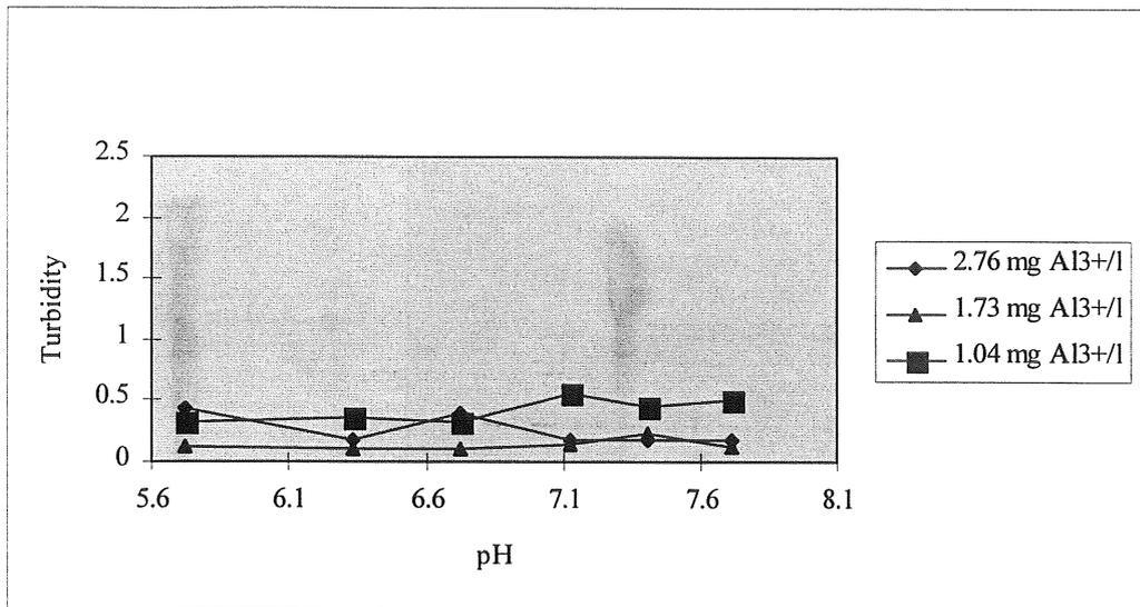
Figure C:5 Effect of dose and pH using PAX XL-60
