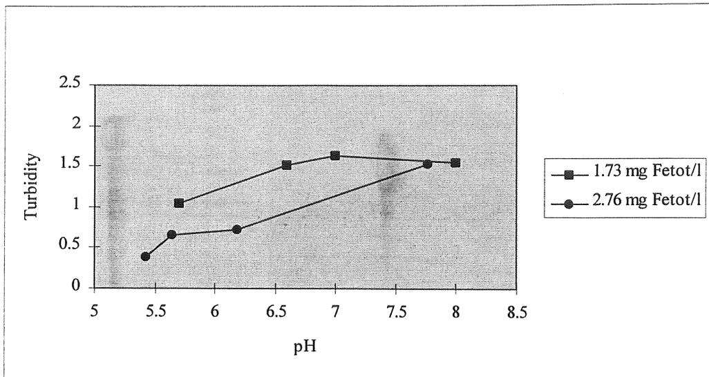
Figure C:9 Effect of dose and pH using FeCl<sub>3</sub>
