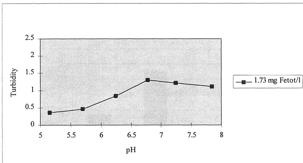
Figure C:8 Effect of dose and pH using PIX 115
