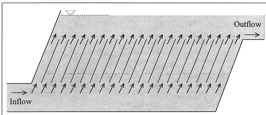
Figure 9:1 Functional separation in tube settler
