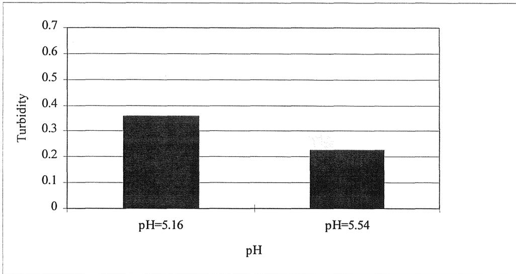
Figure C:17 PIX 115; Turbidity at around optimum pH, dose 1.73 mg  $Al^{3+}$ /l, using different samples of raw water
