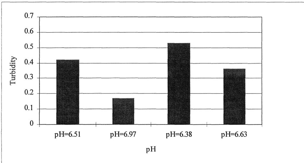
Figure C:12 PAX 16; Turbidity at around optimum pH, dose 1.73 mg  $Al^{3+}$ /l, using different samples of raw water
