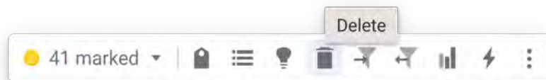
Figure 61. Example of using icons along with tooltips to present options for selected data in a compact and structured way
