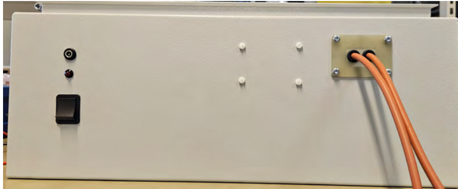
Figure 5.30: Back side UI of the ring wave generator, consisting of a rocker switch with LED, 5 V barrel jack and the high-voltage source connecting wires.
