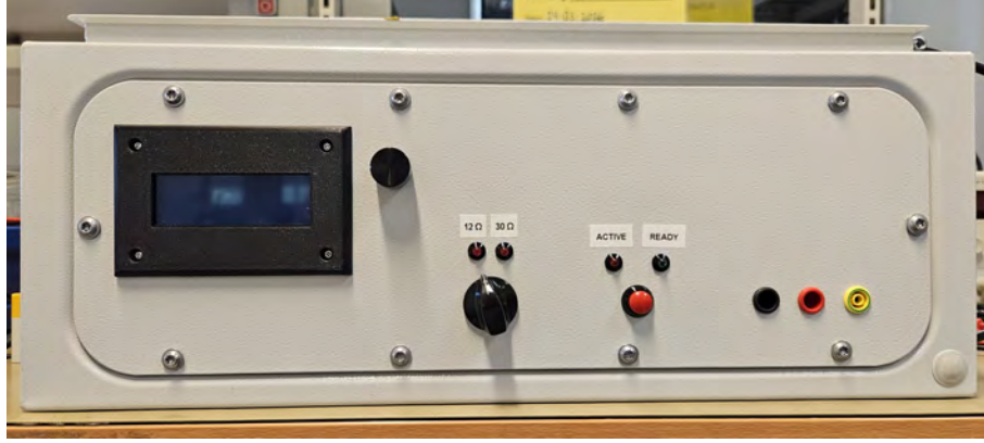
Figure 5.29: Front side UI of the ring wave generator, consisting of an LCD screen, a rotary encoder, rotary switch with LEDs, button with LEDs, and positive, negative and protective earth output ports.
