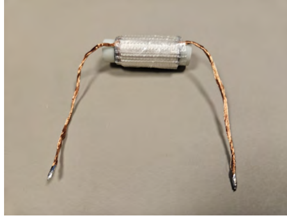
Figure 5.14: Litz wire wound around a fiberglass tube and wrapped with fiberglass tape to make up the 2.7 \mu\text{H} air core inductor, designed for 5 kA.
