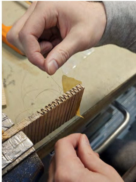
Figure 5.18: Ayrton-Perry winding procedure of the 12 \Omega resistor.
