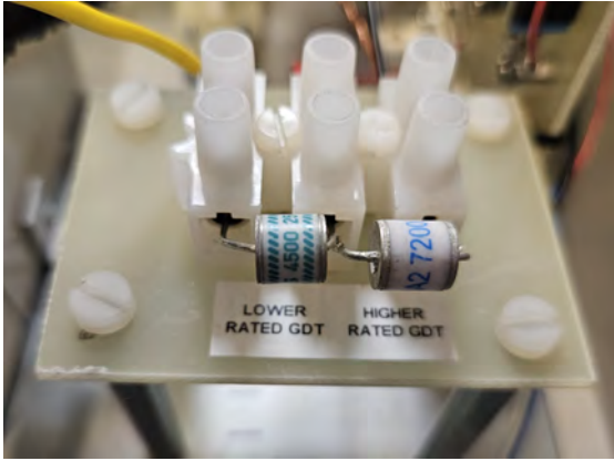
Figure 5.8: View of GDT connections on platform and labels for easier understanding of connections.
