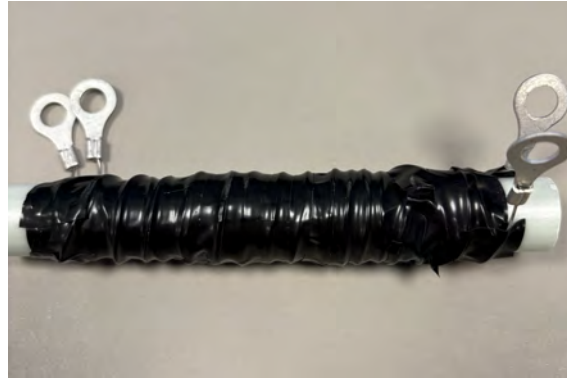
Figure 5.12: The 1.3\ \Omega filter resistor, made from nichrome wire wound around a fiberglass tube using the Ayrton-Perry winding method, and is designed for 10 kV.
