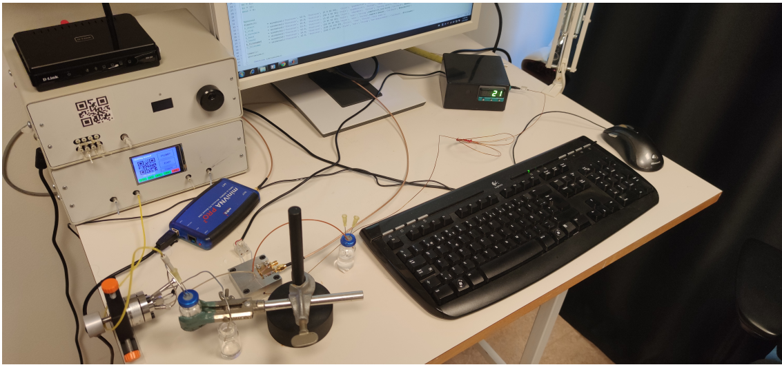
Figure 1.3: Third generation measuring platform: Closed system with metal sensor holder
