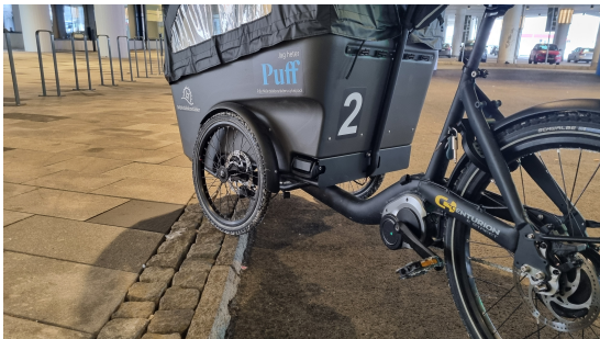
(c) An example of a small bump with a large effect on the comfort of the ride.
