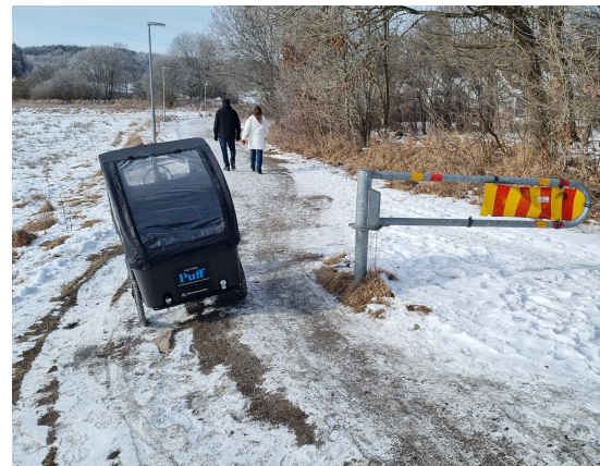
(d) Tilting passage that increased the risk of tipping over the bike.
