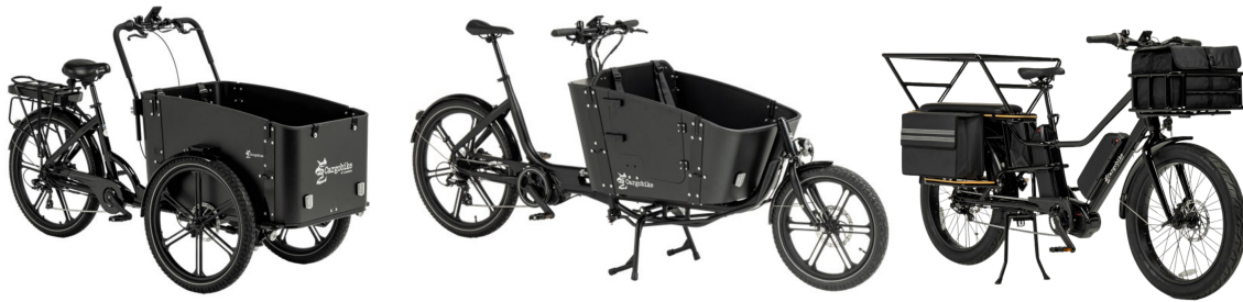
Figure 1.1: Three cargo bike designs that dominate the Swedish market. From the left to the right, the models are commonly called, three wheeled cargo bike, long-john, and long tail.
