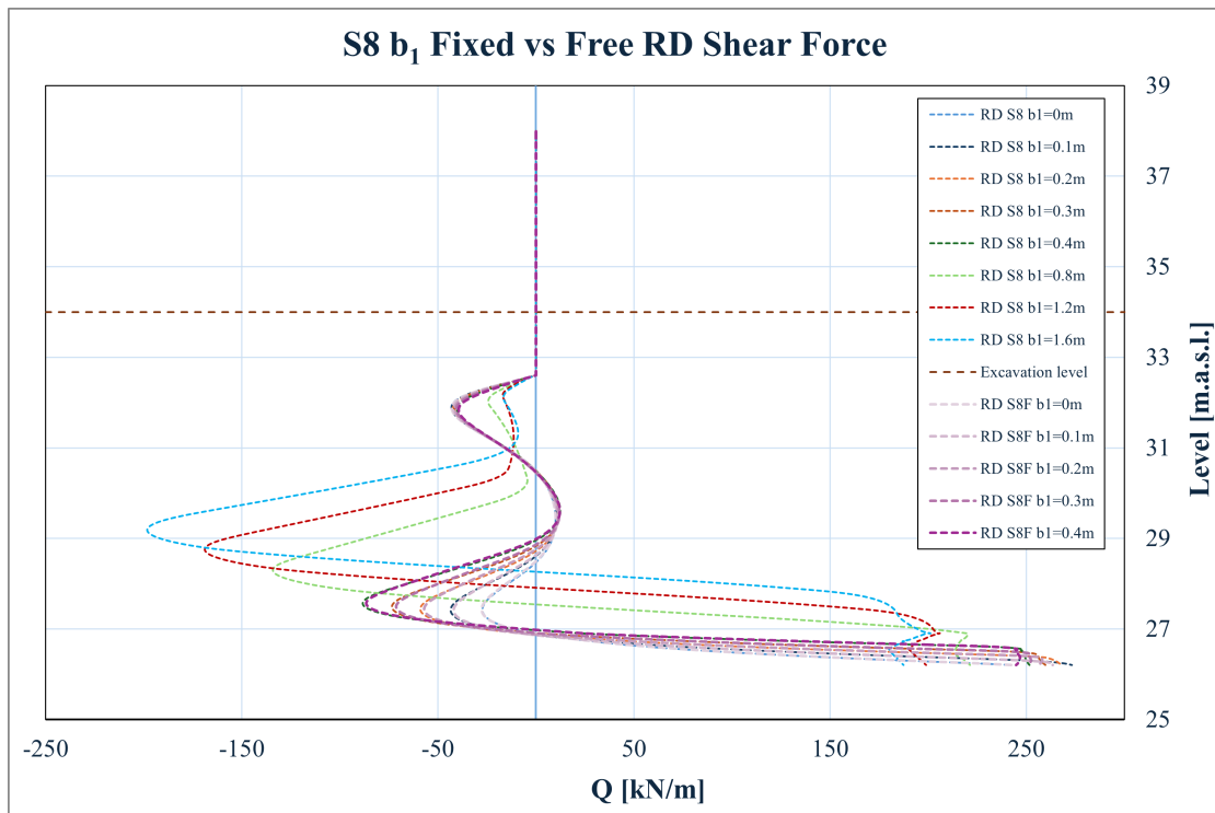
Figure D.5: Section 8 shear force in the drilled pile comparing fixed-end and free-end conditions for variations in b_1 .
