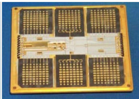
Figure 1.6 Photograph of ASTYX's 77 GHz radar sensor with microstrip patch antenna arrays [14]
