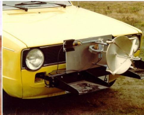
Figure 1.4 An early automotive radar with a parabolic reflector antenna [12]
