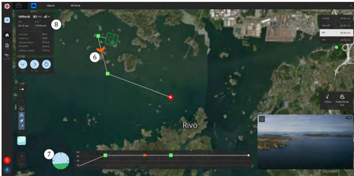
Figure 6.12: The frame during an active flight. The user sees the drone's position in the map and its altitude in the altitude schematics. The camera on the drone's image is visible in the bottom right corner. Numbers in the image are referred to in the text.
