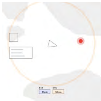
Figure 5.9: Feature for determining the optimal time at scene in combination with time to the target. The border radius of the circle represents how far the drone can travel with the current configuration of ETA and ETS.
