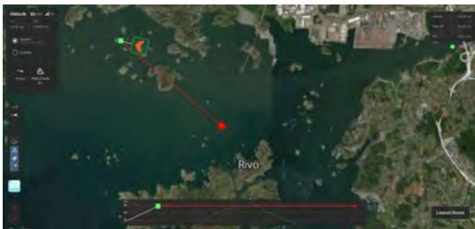
(a) A route has been mapped out by the system. The system alerts the user about the island of larger size between the target and the launcher. The data about the island's ground level informs the user of a collision risk.
