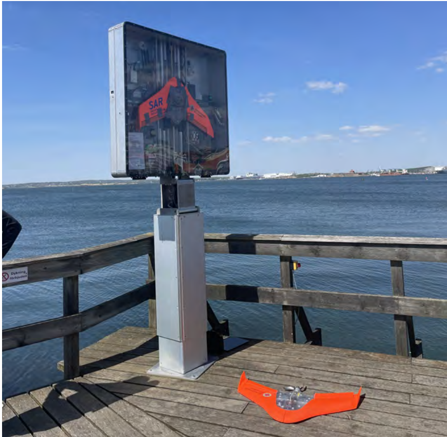
Figure 2.1: The drone developed through the EOS project along with the developed launcher (catapult)
