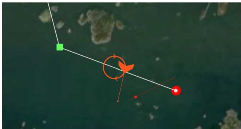
Figure 6.13: When the drone needs to make way for other vehicles, one option is to immediately start loitering. The image shows how the interface informs the user that the drone is loitering.
