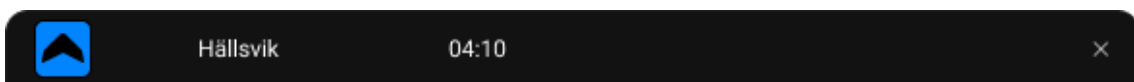
Figure 6.18: A tab leads the user to a more detailed view of a specific flight. The tab itself also contains information in a low level of detail (name of the drone, and estimated time to next waypoint).
