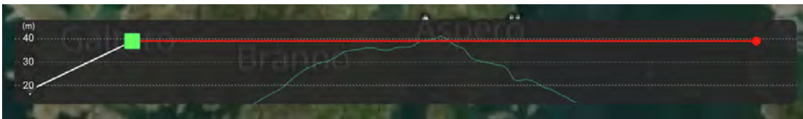
Figure 5.16: Altitude schematics component indicating a risk of collision ahead by marking the route red.
