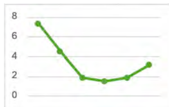
Figure 5.21: A chart of one participant’s mean answering time to the questions in relation to the number of drones they were operating. The first dot represents two drones simultaneously and the last dot represents seven drones simultaneously.
