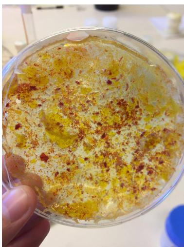
**Figure 3.10:** Showing GPE:AX 4:1 film made with FITC labelled AX
