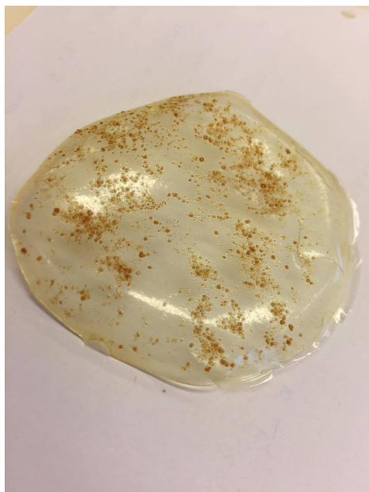
**Figure B.4:** Showing GPE:AX 9:1 made according to procedure 2.1, PU-GPE:AX films.
