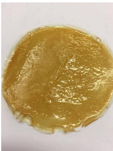
**Figure 3.7:** Showing GPE:AX 4:1 made according to procedure 3.1
