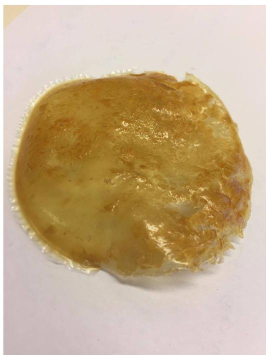
**Figure B.9:** Showing GPE:AX 4:1 made according to procedure 2, homogeneous PU-GPE:AX films.
