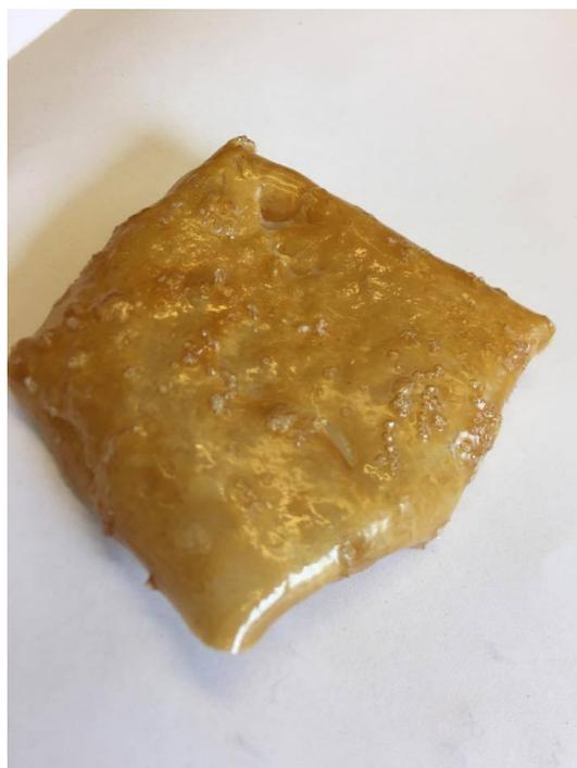
**Figure B.10:** Showing GPE:AX 4:1 made according to procedure 2.1, homogeneous PU-GPE:AX films.
