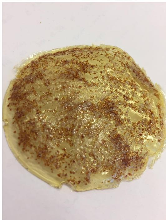
**Figure B.6:** Showing GPE:AX 2:1 made according to procedure 2.1, PU-GPE:AX films.
