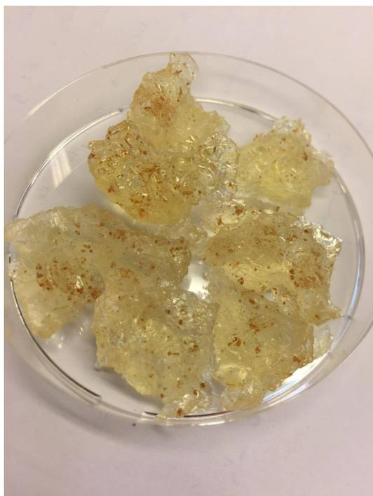
**Figure B.1:** Showing GPE:AX 9:1 made according to procedure 1, PU-GPE:AX films.
