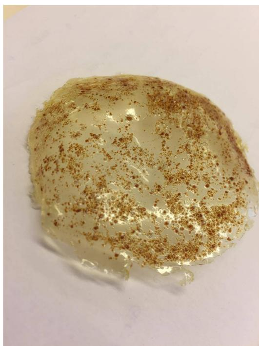
**Figure B.5:** Showing GPE:AX 4:1 made according to procedure 2.1, PU-GPE:AX films.
