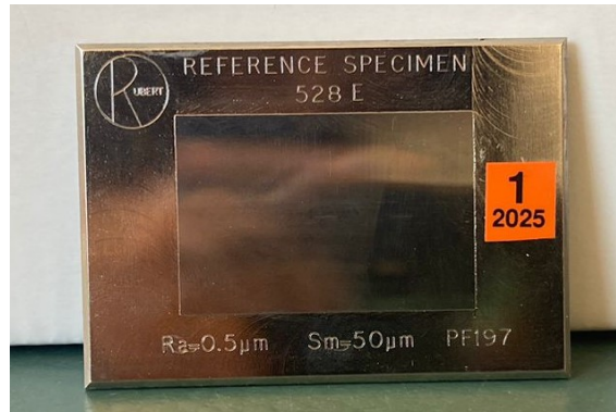
Figure 5.4: Reference specimen for surface Roughness
