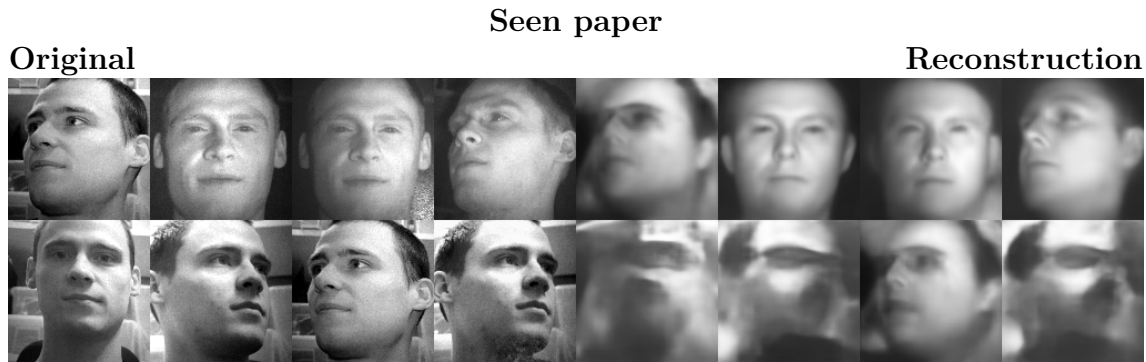
Figure 4.12: Sample reconstructions from the seen paper subset from DCVAE. Images similar in domain to the car interior are reconstructed the best. When the domain changes to a light background the network fails completely to reconstruct.
