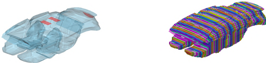
(a) The cabin volume inside GEM3D. (b) The discretized cabin volume in GEM3D.
