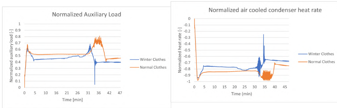
(a) Comparison of the auxiliary load. (b) Comparison of the condenser energy rate.
