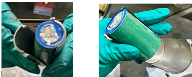
Figure 3.11: Cut open steel casing being pulled wide apart to free the jellyroll
