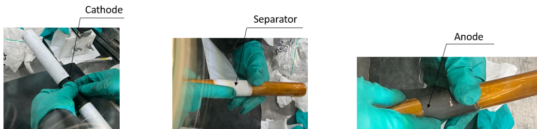
Figure 3.14: Cathode, separator, and graphite anode being wound over cylindrical tubes, respectively
