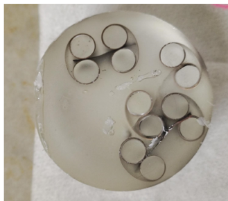
Figure 3.17: Epoxy cast removed from the plastic mould
