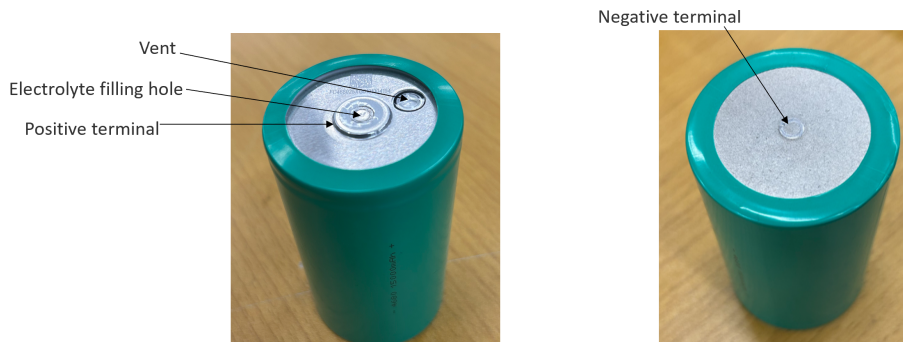
Figure 3.1: Figure depicting the positive and negative terminals of the T.O
