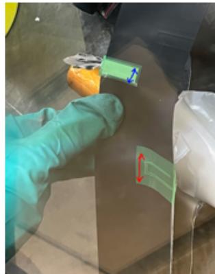
Figure 4.3: Broad and narrow green plastic films on the cathode side
