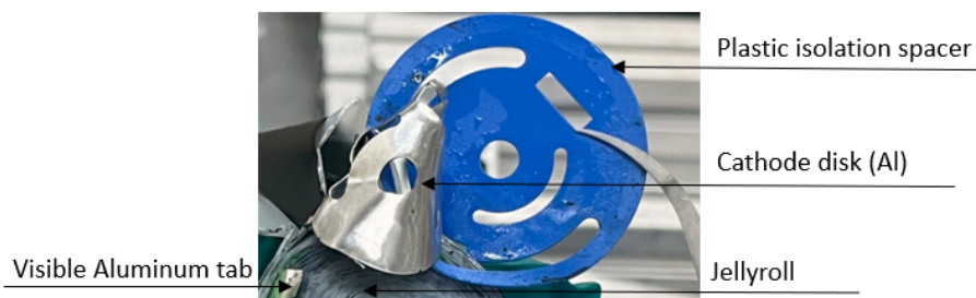
Figure 4.16: The blue plastic isolating plate can be seen underneath the cathode disc
