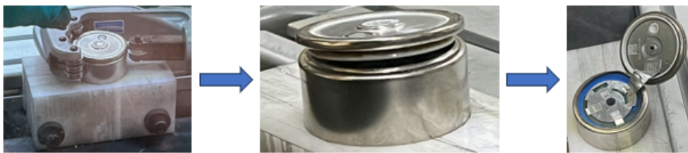
Figure 3.3: Using a pipe cutter the positive cap as seen in Figure 3.1 was opened to reveal the plastic ring separating the Al tabs from the casing
