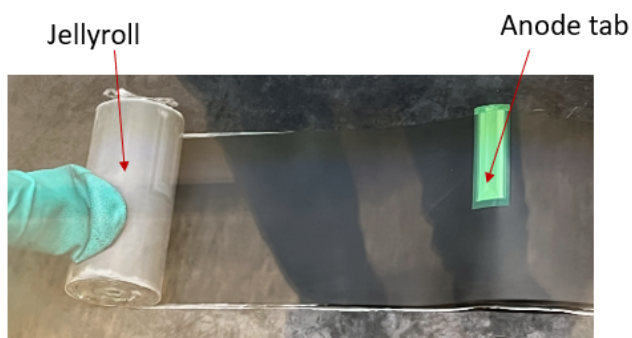
Figure 3.13: Jellyroll being unwound for measuring the length of electrodes
