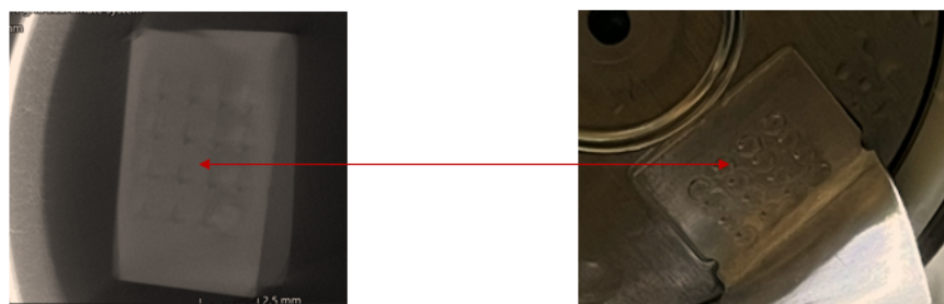
Figure 4.21: Cathode disc laser welded onto the positive terminal
