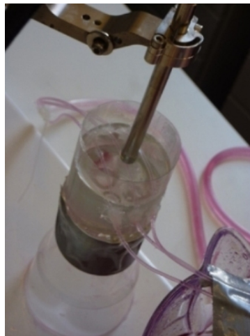
Figure 3.4: Dielectric Probe in close contact to the blood vessel phantom.
