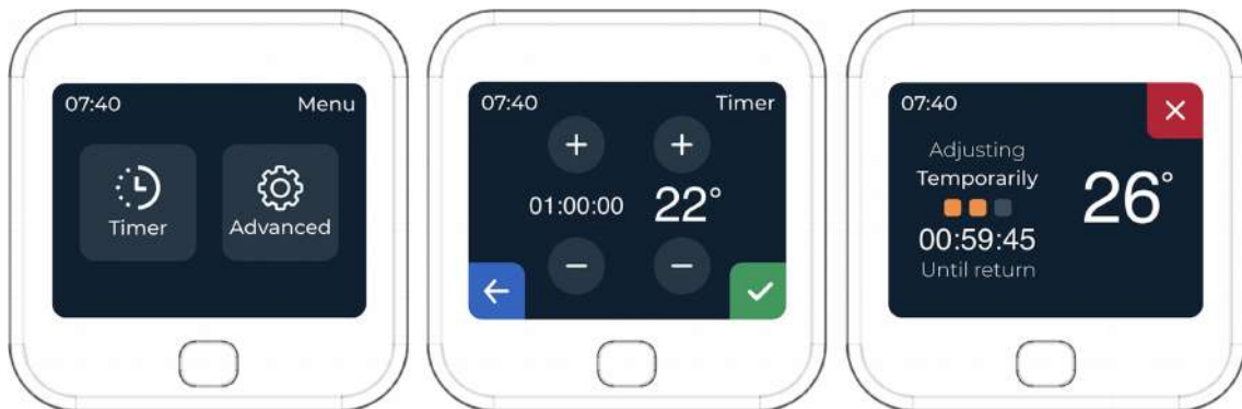
Figure 7.11: Thermostat menu, timer setup and main screen during timer. [Authors own image]
