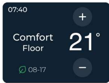
Figure 7.24: The comfort temperature set to recur as 21° during the week
