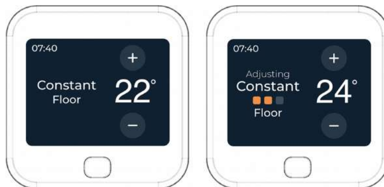
Figure 7.9: Thermostat main screen in constant mode. [Authors own image]
