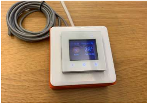
Figure 6.2: A competitor thermostat in the 3D printed testing rig. [Authors own image]
