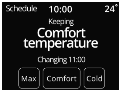
Figure 7.17: Early prototype that only uses 3 thermal presets, max, comfort and cold
