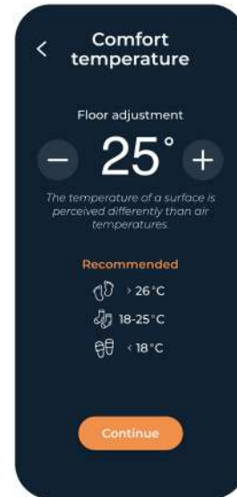
Figure 7.16: Set up suggestions for picking comfortable floor temperatures
