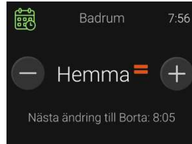
Figure 7.18: Early prototype that used a bar scale ranging the steps over or under a thermal baseline called Home ("Hemma")
