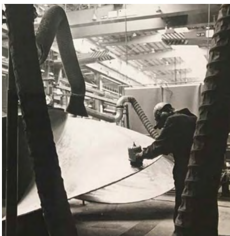
Figure 3. Worker grinding ship's turbines in the warehouse.
