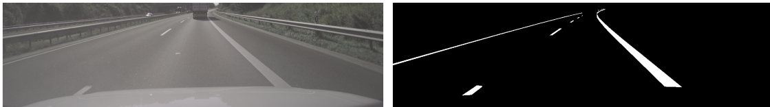
Figure 3.8: Example sample of the Lane dataset. To the left you find the input image and to the right the ground truth segmentation mask.
