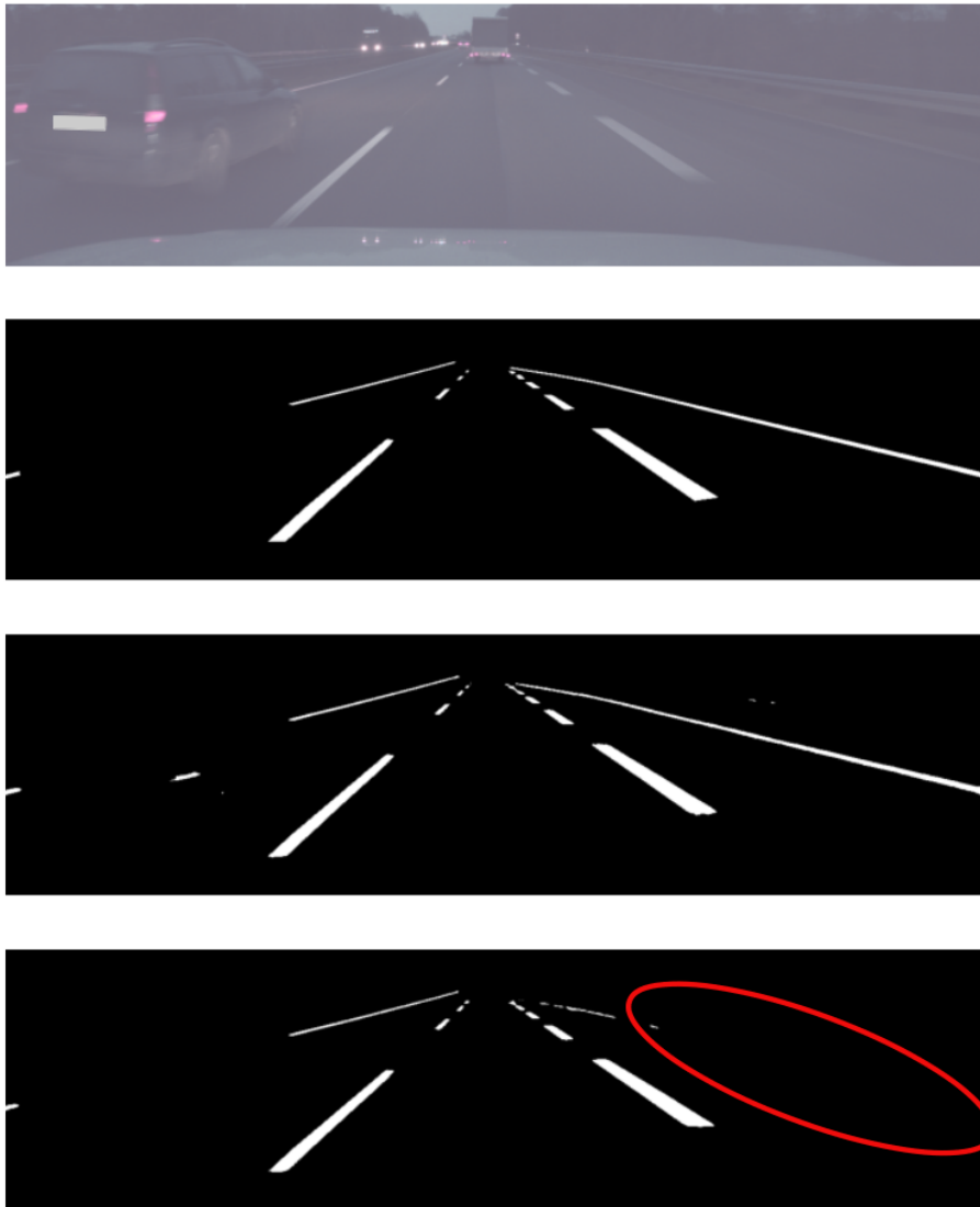
Figure 4.8: Top picture – input image. Second from the top - target image. Second from the bottom – prediction made by the smallest baseline model. Bottom picture – prediction made by the smallest attention-augmented model. Note that in this case the attention-augmented model misses a lane that is picked up by the baseline.
