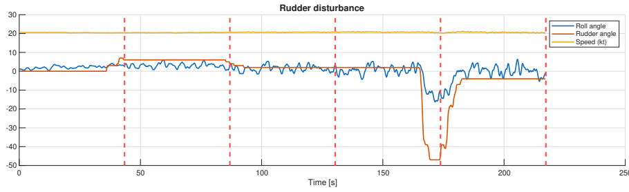
Figure 5.12: The rudders effect on roll angle and speed in the RAMP dataset, the vertical red dashed lines indicates the time where the periods end and transition to a higher amplitude. A large rudder disturbance is recorded at the end of period 4.
