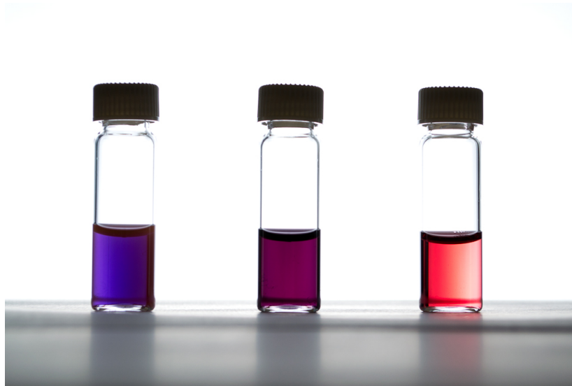
Figure 2.2: Colloidal dispersion of gold nanoparticles in water, displaying varied colors due to their size-dependent plasmonic resonance. [19]
