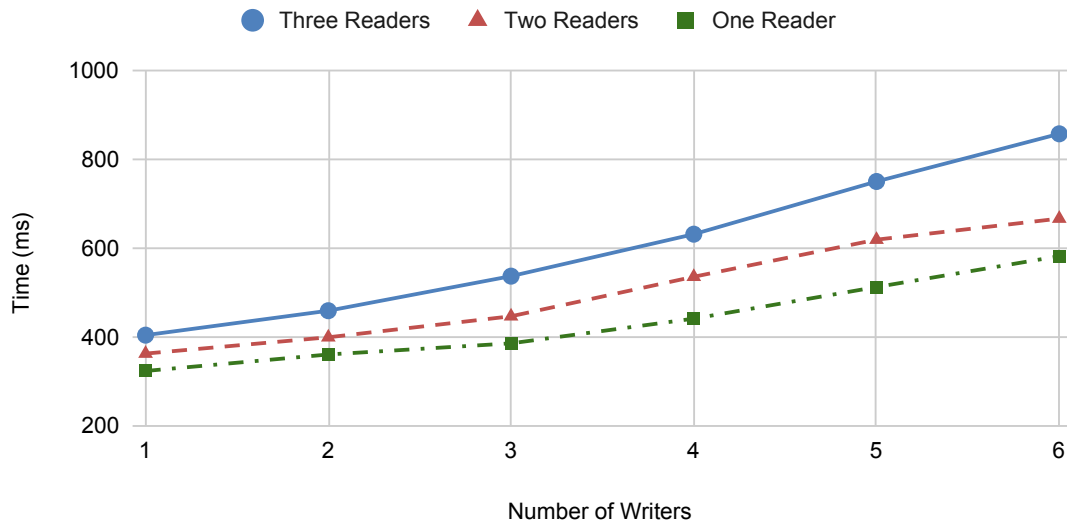
Figure 7.9: Average latency of performing different emulation operations with a constant number of readers and a varying number of writers
