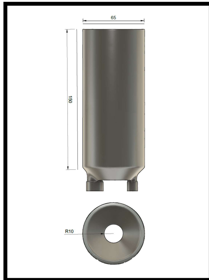
Figure 1.1. The dimensions of the heat exchanger from Bättre Design (Dybeck, 2023).
