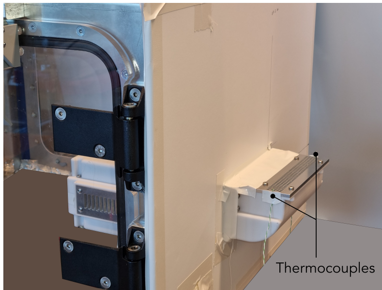
Figure 4.3: Positioning of the test unit at the entry of the wind tunnel.
