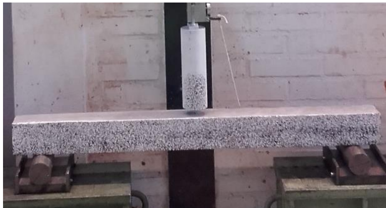
Figure 7.4 Setup for impact loading tests. Note the back and white speck pattern painted on the beam surface and the drop-weight.
