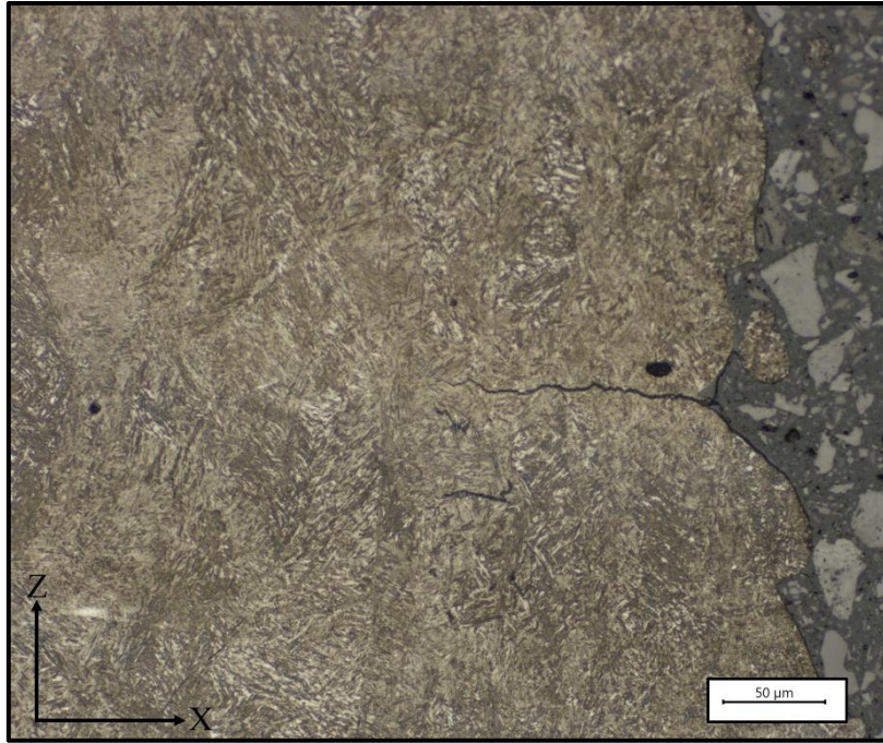
Figure 13. Surface crack propagating perpendicular to the build direction in a cross-section of 4140 steel.
