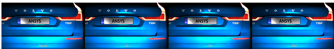
Figure 5.16: Anti aliasing in detail. From left to right is None, 2×, 8× and 16×
