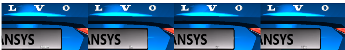
Figure 5.17: Anti aliasing in detail. From left to right is None, 2×, 8× and 16×. Zoom in to the line of the model shape.
