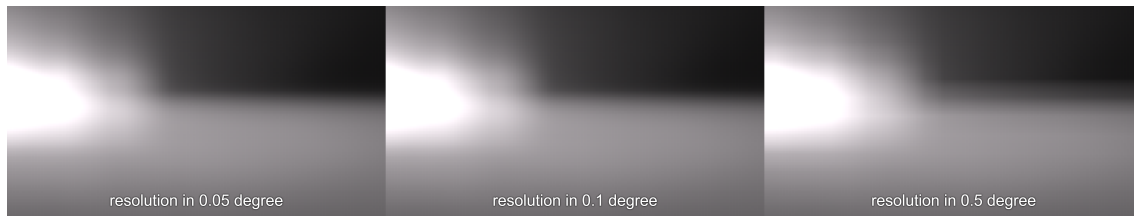
Figure 5.11: Renderings of the same light pattern in AVxcelerate with different sampling resolutions. A smaller angular step ( 0.05^\circ ) yields a sharper and more precise edge compared to the coarser 0.1^\circ sampling.
