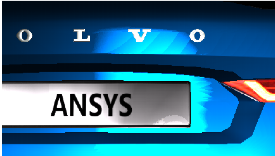
Figure 3.6: A topical aliasing photo. Notice that there are artifact patterns close to Volvo letter.
