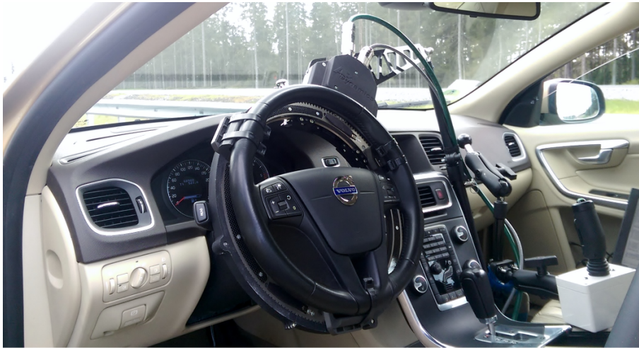
Figure 7.2: SR 60 Orbit steering robot mounted in the test vehicle
