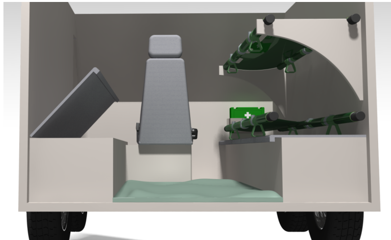
Figure 25: Vehicle layout with open bench for CasEvac mission 1B
