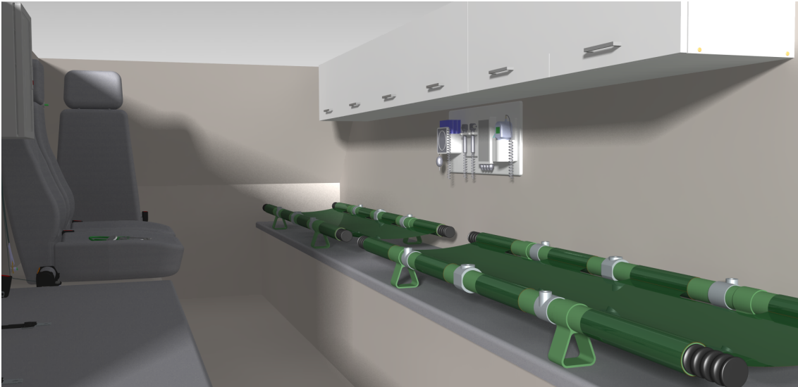
Figure 28: Internal layout with stretchers and enclosed storage compartments for MedEvac mission 2B
