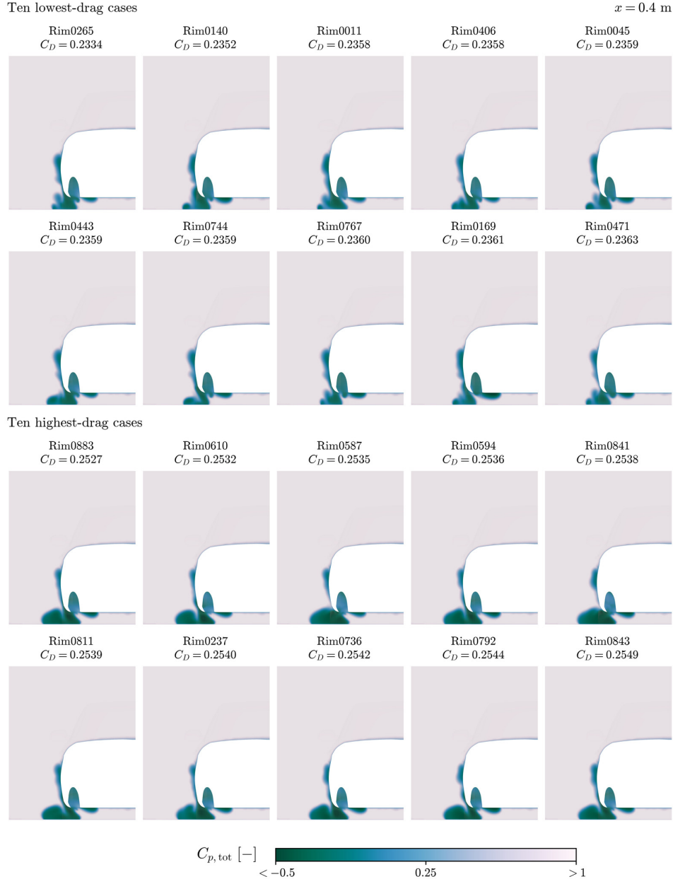
Figure 5.21: Mean total pressure coefficient downstream of the front wheel at x = 0.4 m. Case order, crop, and colour scale match Figure 5.20.
