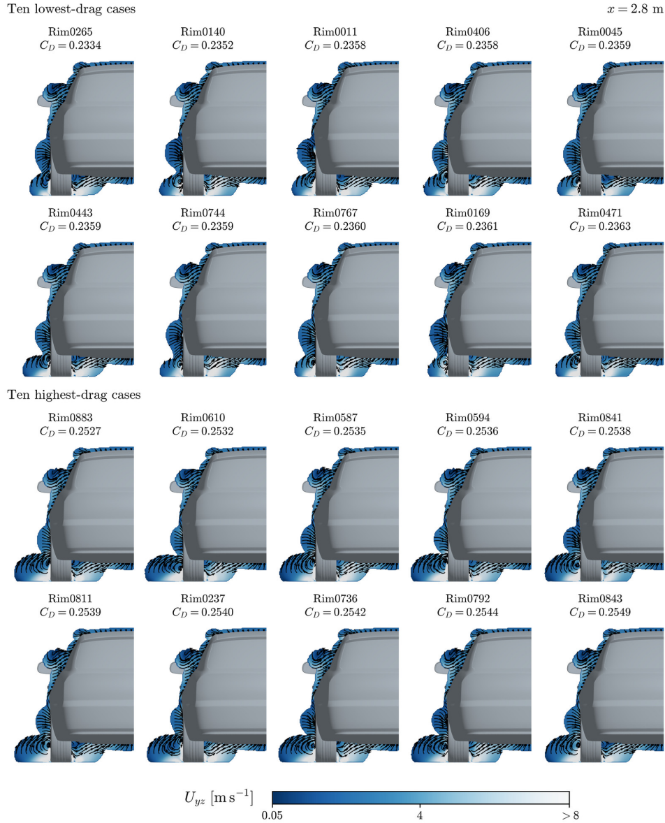
Figure 5.22: Mean crossflow at x = 2.8 m, ordered as in Figure 5.20. Arrows indicate direction, and colour gives U_{yz} from 0.05 to 8 m s -1 , within the C_{p,\text{tot}} < 0.9 mask.
