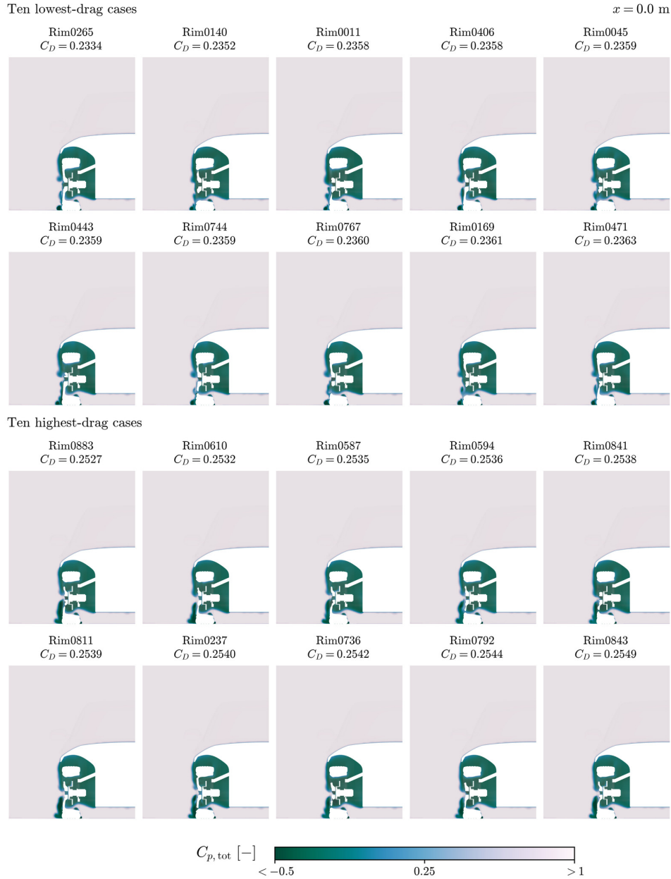
Figure 5.20: Mean total pressure coefficient at the front wheel centre, x = 0 . Upper two rows: ten lowest drag cases. Lower two rows: ten highest drag cases. Each group follows increasing C_D . The left half of the view is shown, with -0.5 \leq C_{p, \text{tot}} \leq 1 .
