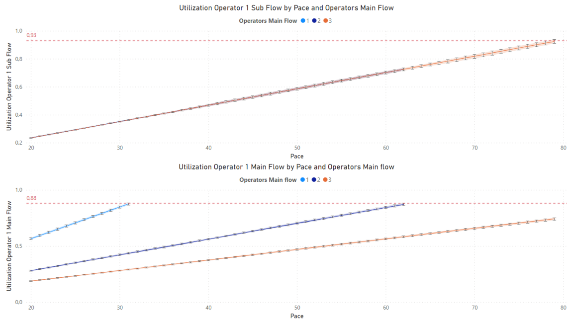
Figure 4.5: A line plot illustrating the average Worker Utilization rates for an assembly worker at the main flow and sub-flow as a function of pace.
